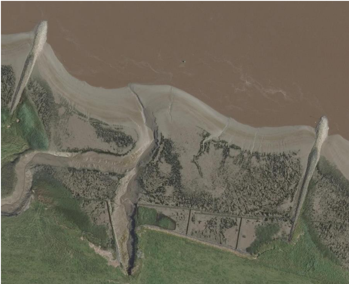
Aerial photograph of the brushwood boxes built between groynes no. 7 and 9.
