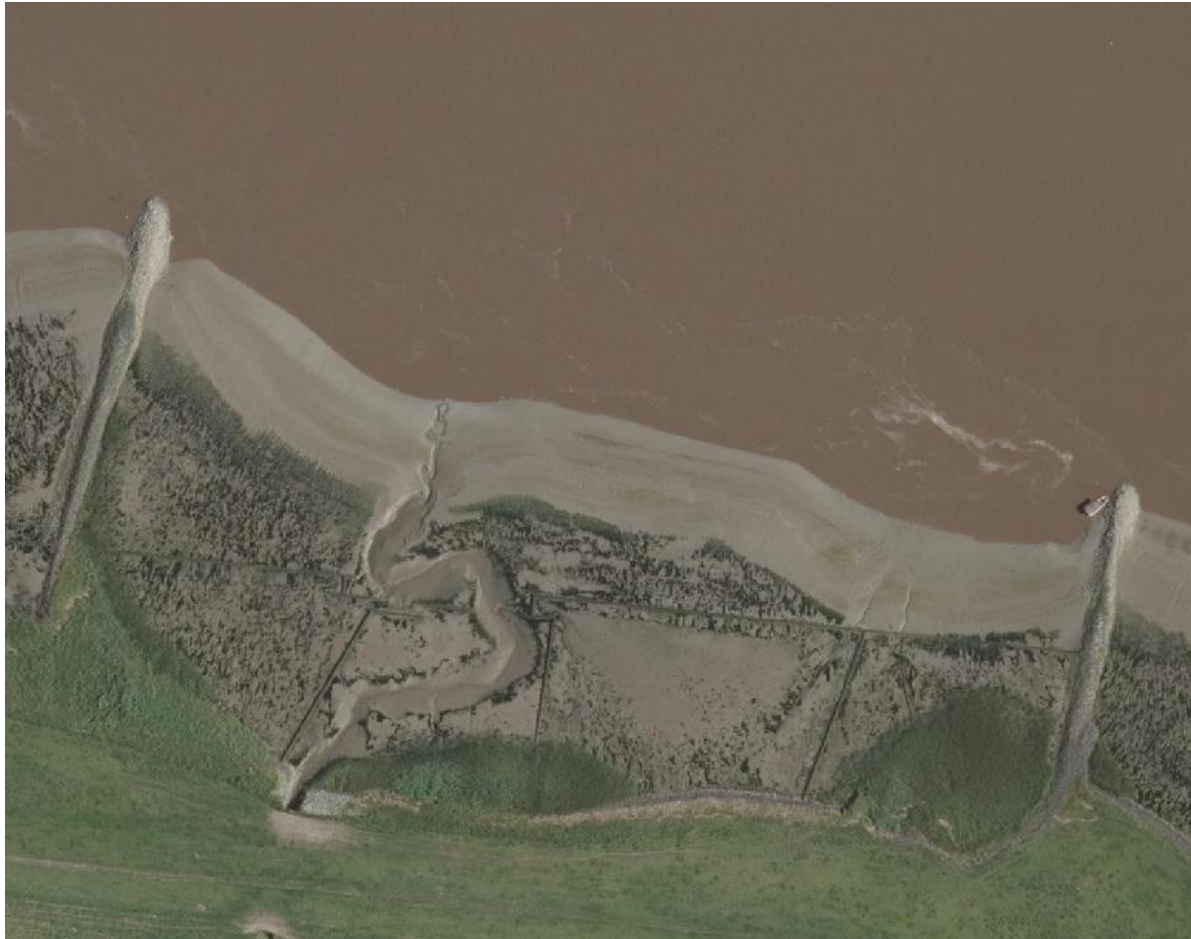
Aerial photograph of the brushwood boxes built between groynes no. 9 and 11.
