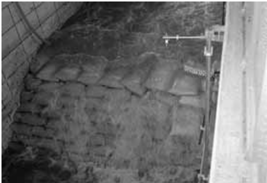
Figure 5. Large-scale model tests with geotextile containers
