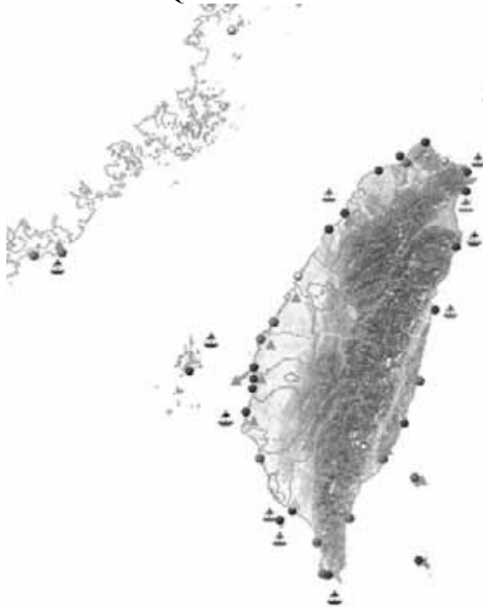
Figure 1. The real-time and in-situ measurement network around Taiwan. The buoy-like symbol is the locations of data buoys. Circle symbol represents the tide stations. Triangular symbol represents the coastal weather stations.
