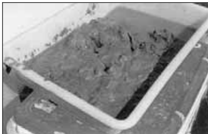
Figure 5 - Sediment extracted near the Ribarroja's dam, currently being studied for use to reduce problems of subsidence in the Ebro Delta.
