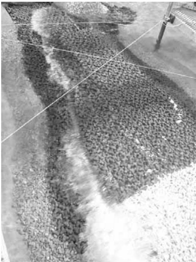
Figure 3. 3D physical model tests on hydraulic stability (1/69 scale): top view of the immersed tunnel, ACCROPODE™ II armour layer.
