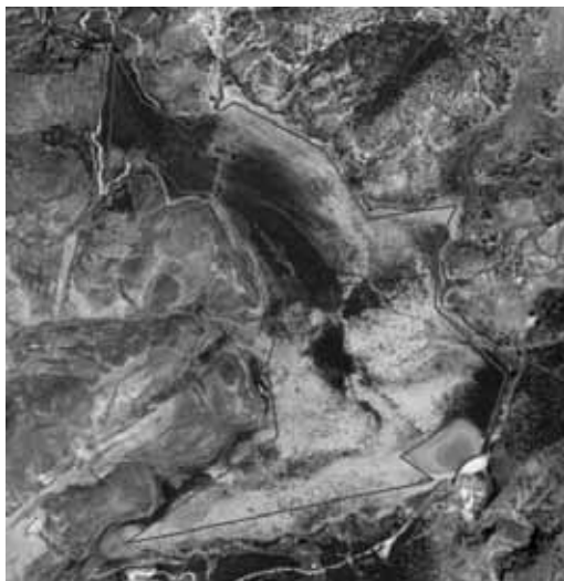
Figure 1: Valdeinferno reservoir (Initial capacity: 25 hm 3 ; Volume of sediment accumulated: 14 hm 3 )
