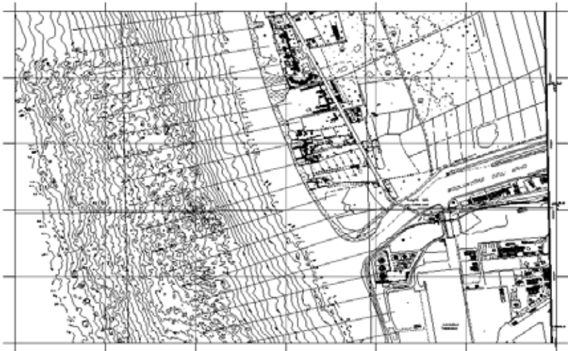
Figure 9 : Real bathymetry detected by multibeam survey (2006) shows that the southern part of Pisa littoral is characterised by bedforms (about 20-30 cm of amplitude) which disappear moving toward north
