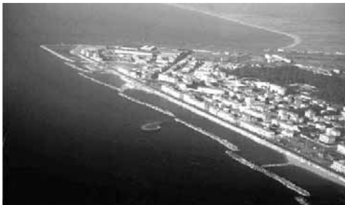
Figure 1. Marina di Pisa, Tuscany, Italy. The defense of the coast on the left side of Arno river mouth has been assured by emerged rubble-mound breakwaters since 1938. On the opposite, the right side of the coast is unprotected and has been
