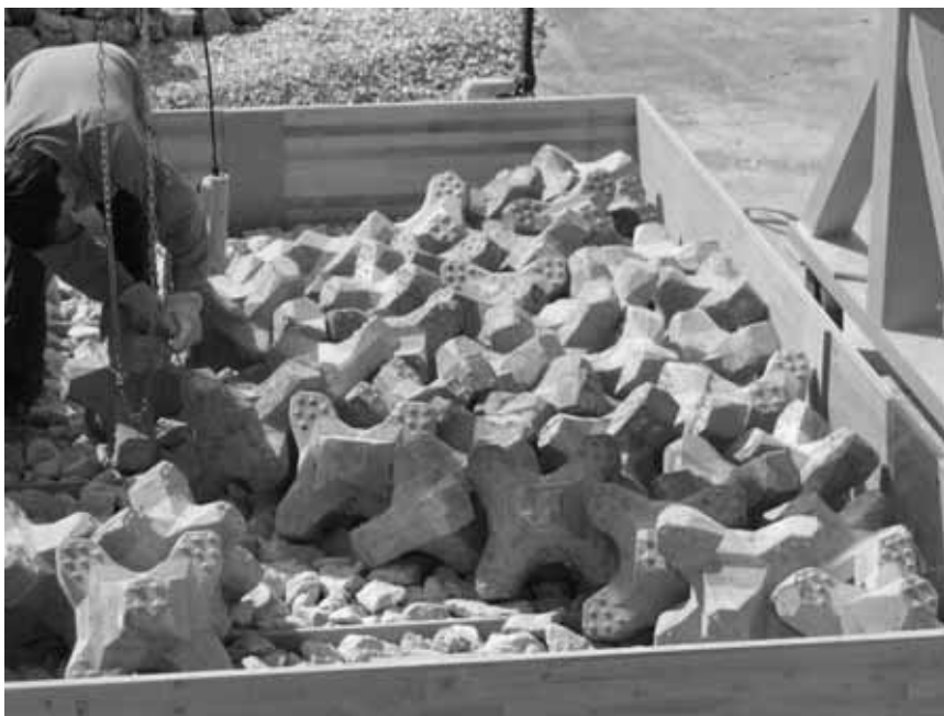
Figure 1. Dry tests on armour unit placement (~1/8, 1/10 scale): tests on 35 kg ACCROPODE™ II units.
