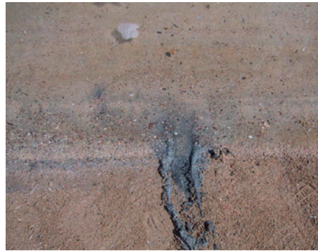
Figure 7. Examples of anoxic conditions and the formation of hydrogen sulphide at protected artificial beaches. Left: Dark substance suspended in the water when seabed at shallow water is disturbed, artificial beach in lagoon environment at the Egyptian NW coast. Right: Dark substance at beach in artificial lagoon in the Red Sea.
