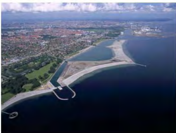
Figure 20 Aerial photo of Amager Beach Park, which consists of the following main elements: island with terminal structures north and south and a separating headland between the northern and southern beaches and a lagoon.
