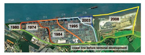
Fig. 3: Development stages of Container Terminal Bremerhaven
