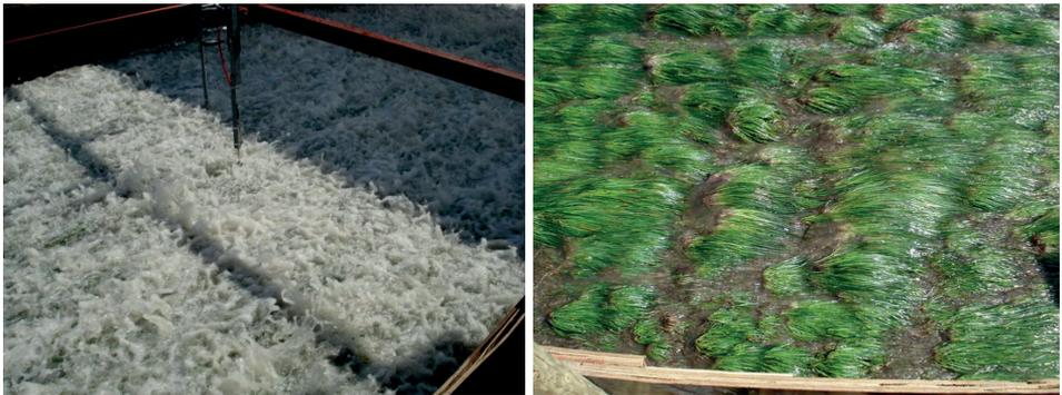
Figure 1: Inner slope of a dike in Delftzijl during in situ overtopping tests.
