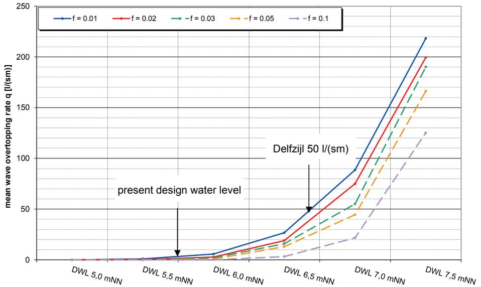
Figure 6: Mean Overtopping rates for different design level scenarios and roughness factors.
