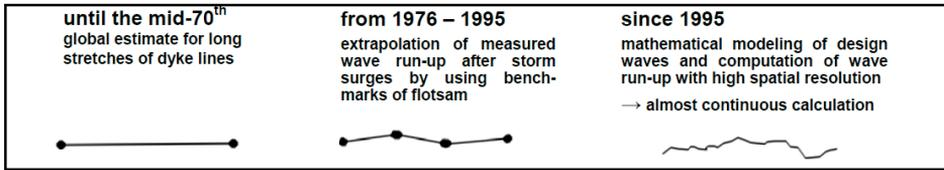
Figure 2: Changes in the evaluation of design wave run-up in Lower Saxony within the last decades (NIEMEYER et al. 2010).
