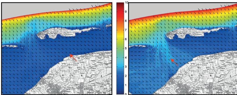
Figure 5: Significant Wave Heights [m] modeled by SWAN (left panel: supposed design water level: 5 m above German datum, right panel: anticipated design water level: 7.5 m above German datum) (BERKENBRINK et al. 2010).
