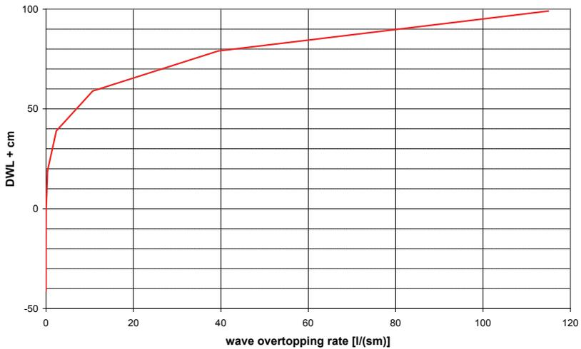
Figure 10: Cumulation of acceptable design water level increase in dependence of overtopping tolerance for an estuarine dike (NIEMEYER et al. 2010).
