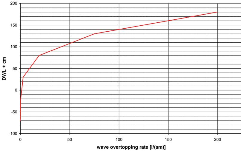
Figure 9: Cumulation of acceptable design water level increase in dependence of overtopping tolerance for an exposed coastal dike (NIEMEYER et al. 2010).
