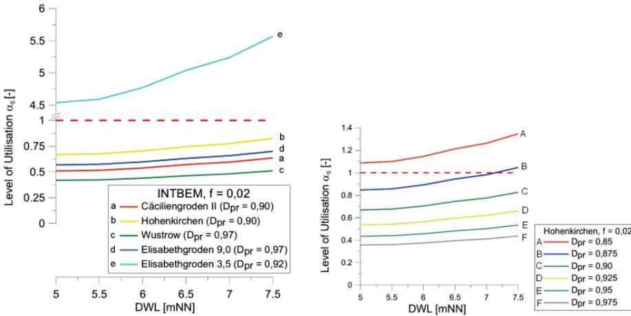
Figure 8: Safety against slope parallel sliding for different types of soil (RICHWIEN et al. 2010).
