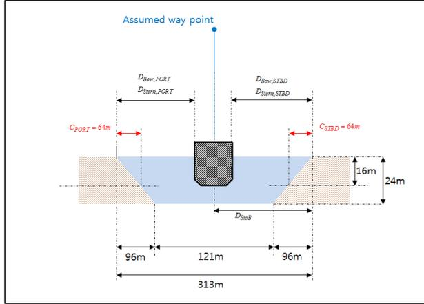
**Figure 3. Design section of the Suez Canal**
