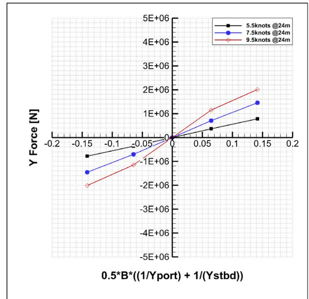
**Figure 7. Calculated Y forces according to the ship location in the Suez Canal**
