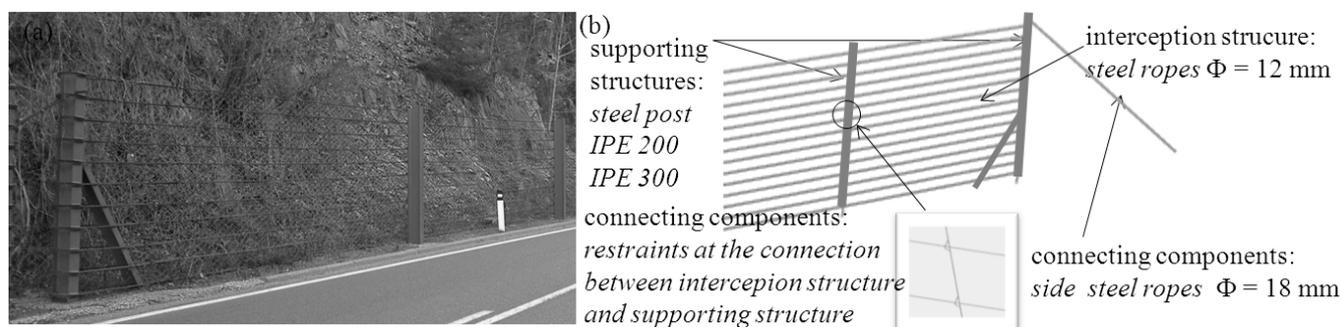
Figure 4. Example of falling rock protection barriers installed in the Autonomous Province of Bolzano: a) barrier ss38\_12\_1 belonging to type ANAS and b) scheme of the functional module of barrier type ANAS.
