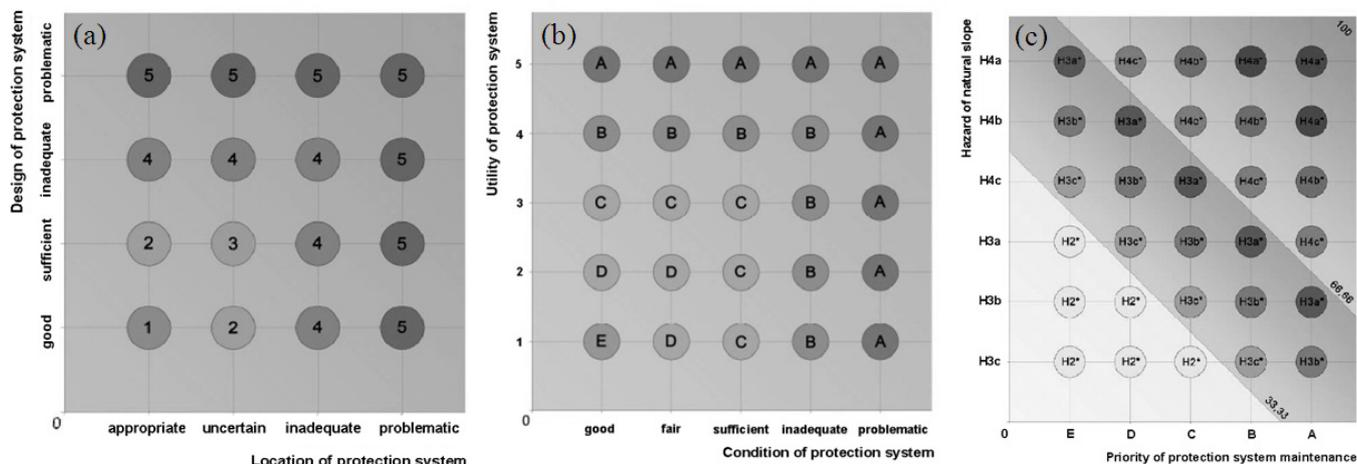
Figure 2. Procedure for the evaluation of the modified hazard  $H^*$ : a) chart for the assessment of the protection system ‘utility’ b) chart for protection system ‘maintenance priority’ and c) chart for the evaluation of the modified hazard  $H^*$ .
