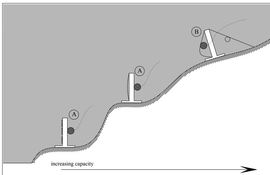
Figure 3. Falling rock protection barrier: scheme of relevant typologies of falling rock protection barriers: A semi-flexible, B flexible.
