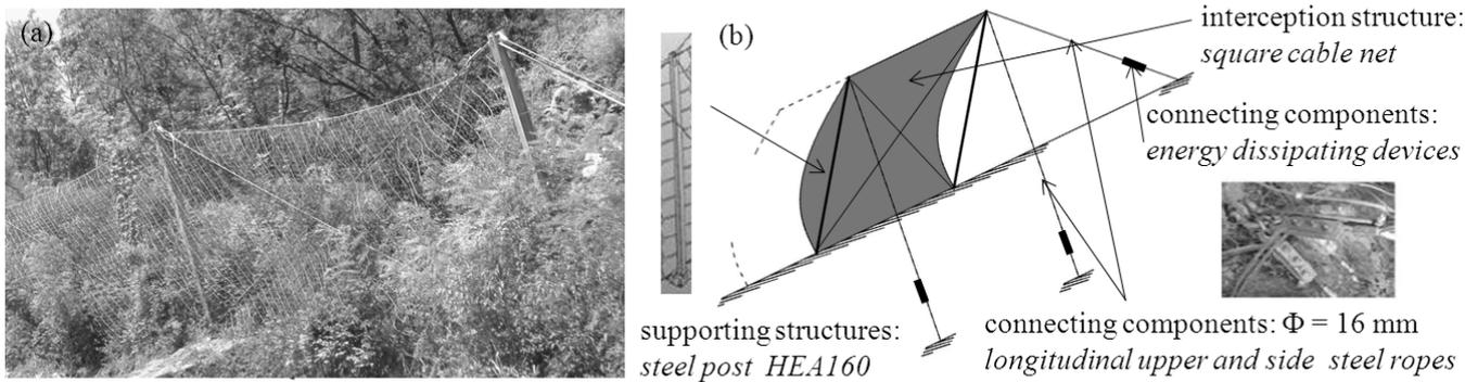
Figure 5. Example of falling rock protection barriers installed in the Autonomous Province of Bolzano: a) barrier 12\_5\_GR\_008/014 belonging to type PT\_B750 and b) scheme of the functional module of barrier type PT\_B750.
