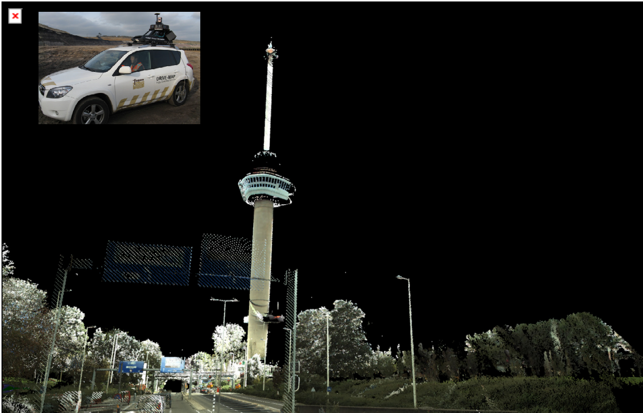
Figure 2. High quality terrestrial LiDAR data acquisition with DRIVE-MAP
