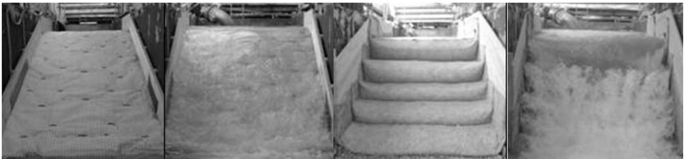
Figure 5. Loaded and unloaded dyke models with slope parallel geosynthetic layers using anchors for fixation (left) and wrap-around method (loops) (right) (Haselsteiner et al., 2008)
