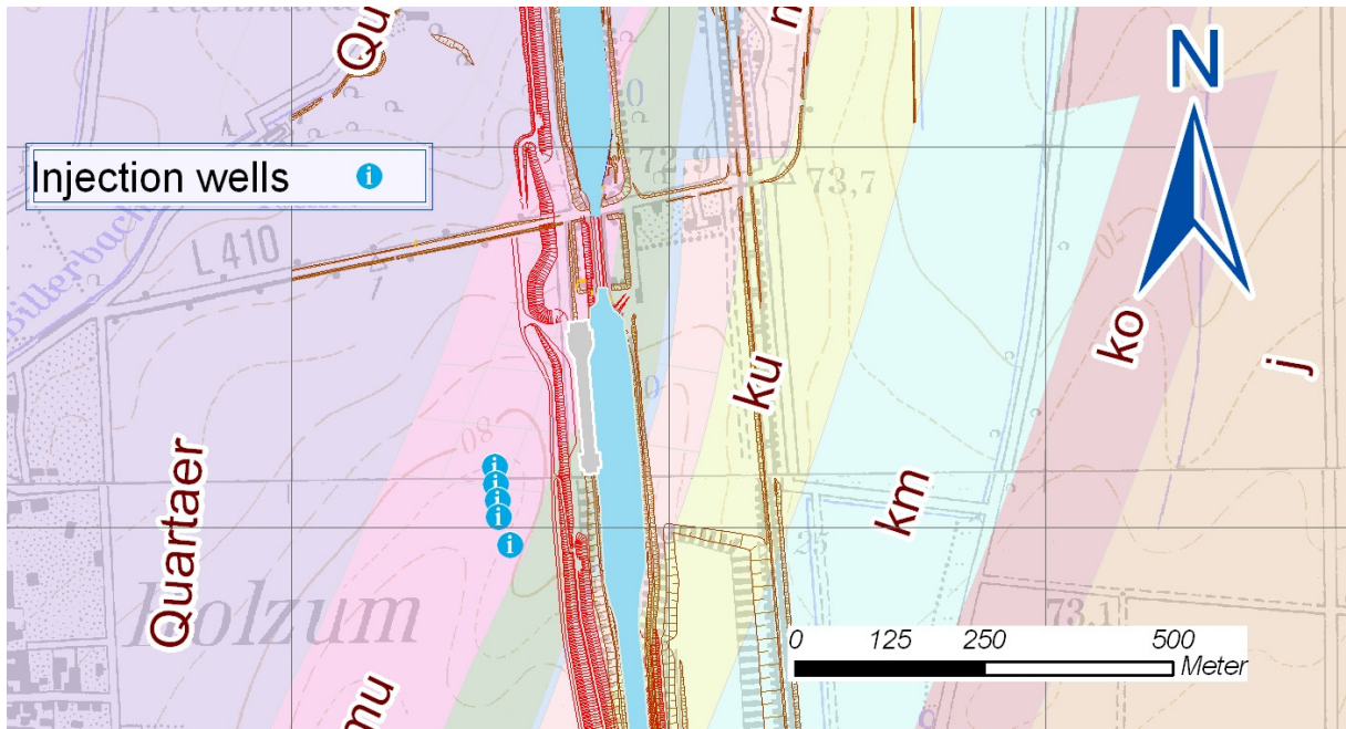
Figure 7. Location of infiltration wells which are to prevent inflow from a southern direction
