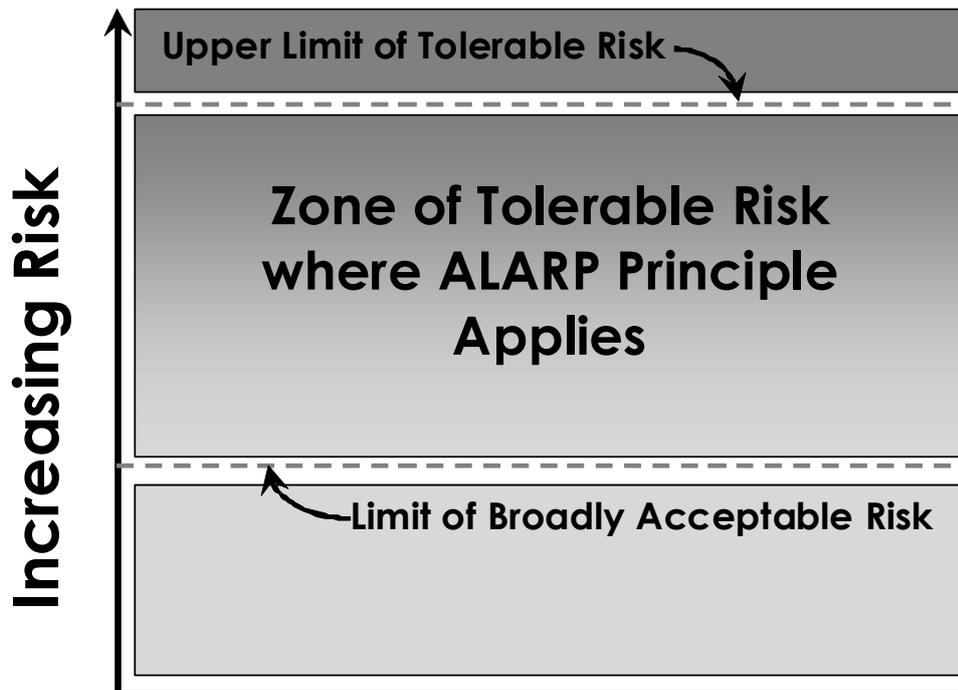
Figure 1. Tolerability of risk and the ALARP principle
