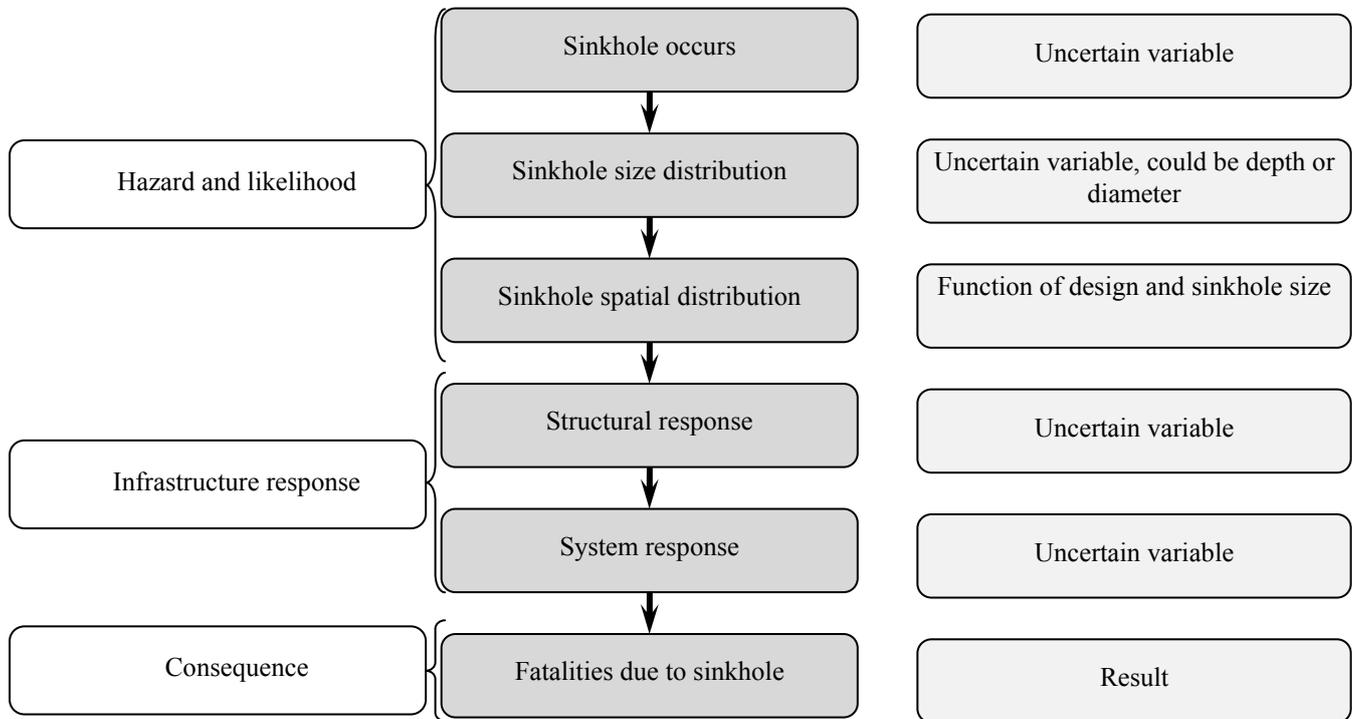
Figure 2. Example risk model for QRA for the sinkhole effect on infrastructure
