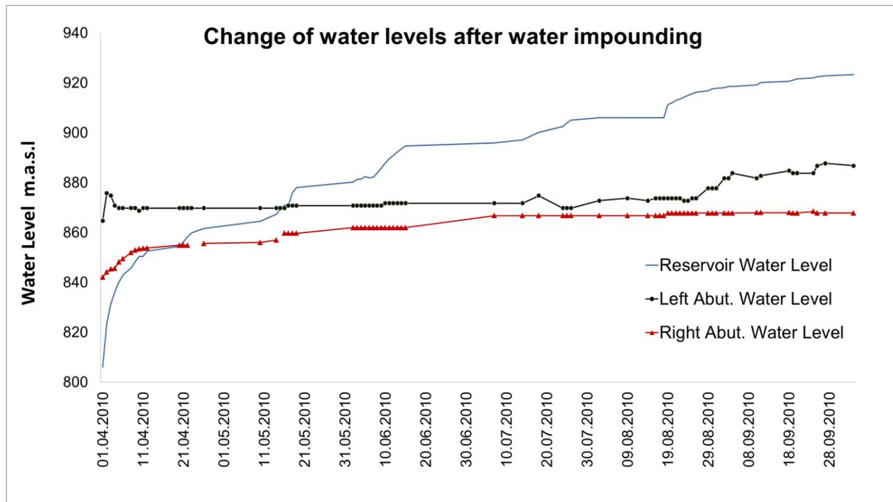
Figure 4. Change of water levels after water impounding of Karun 4 dam (2010)
