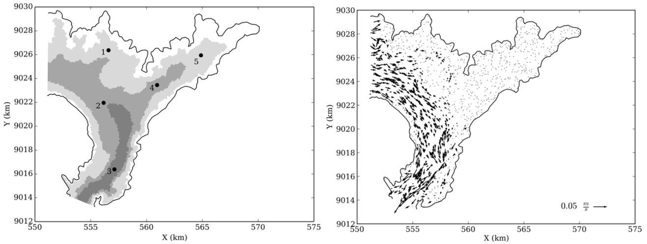
Figure 2. Surface flow simulation for mean flow conditions: control points (left); surface flow simulation without the action of the wind, reference case (right).
