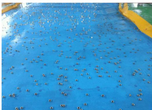
Figure 2. Roughness Adjustment with Block Placement.
