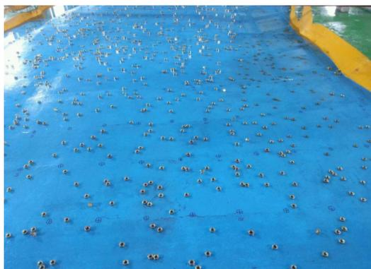
Figure 2. Roughness Adjustment with Block Placement.
