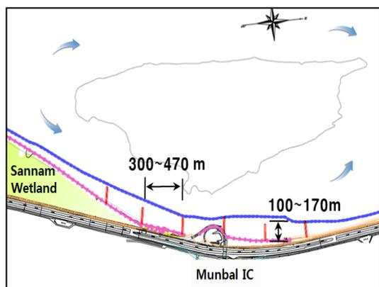
Figure 3. Spur-Dike Arrangement and Dimensions.
