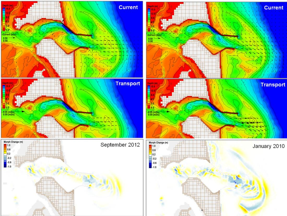
Figure 9. Residual current, sediment transport and morphology change for September 2012 and January 2010.
