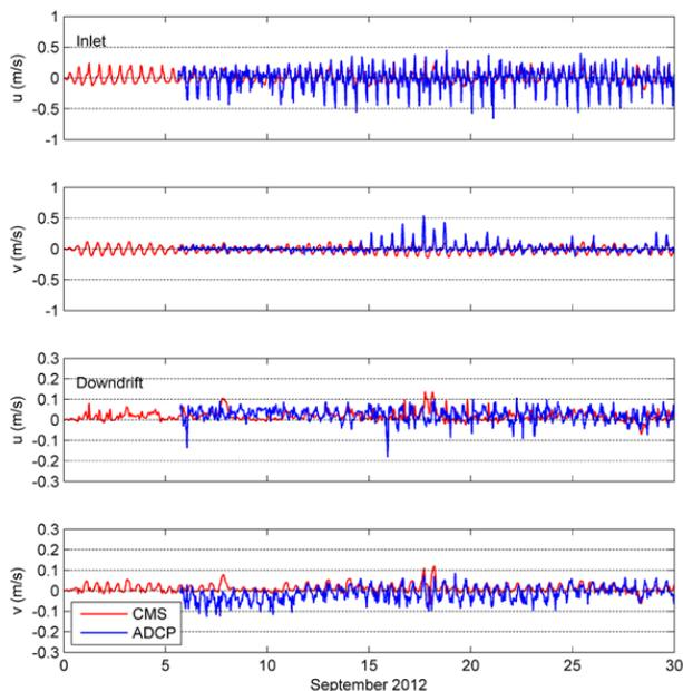
Figure 8. Calculated and measured currents in Merrimack Inlet.
