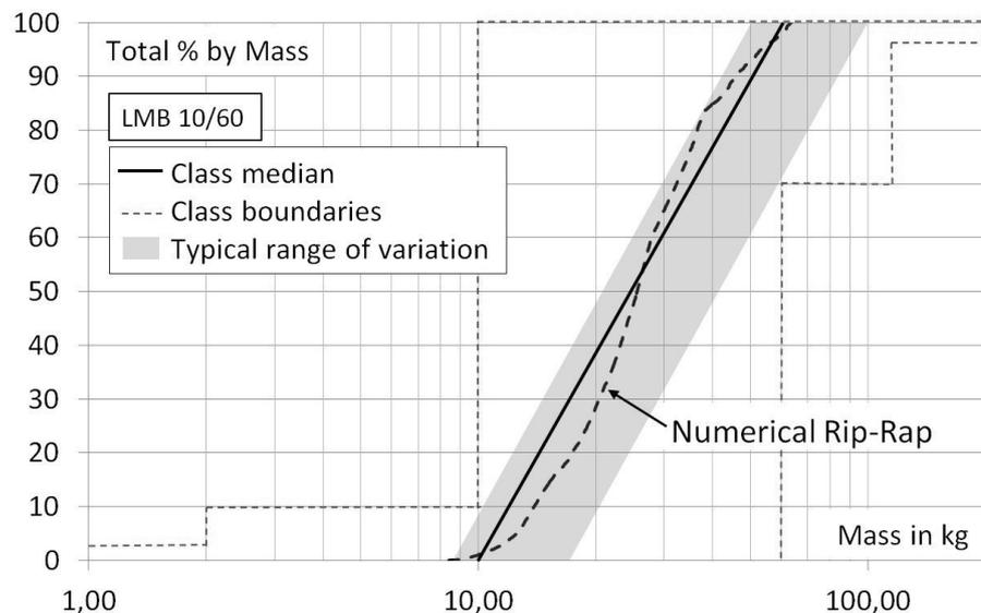
Figure 3. Typical range of variation of cumulative curve for armourstones class LMB<sub>10/60</sub> (BAW 2008), cumulative curve of corresponding numerical rip-rap.
