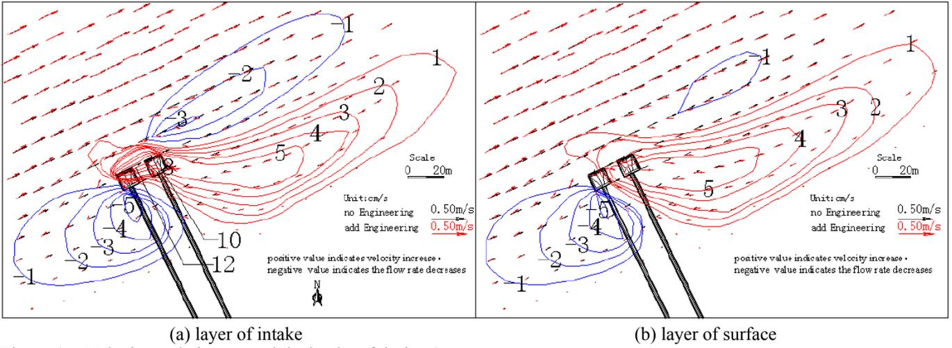
Figure 4. Velocity variation around the intake of design 2.
