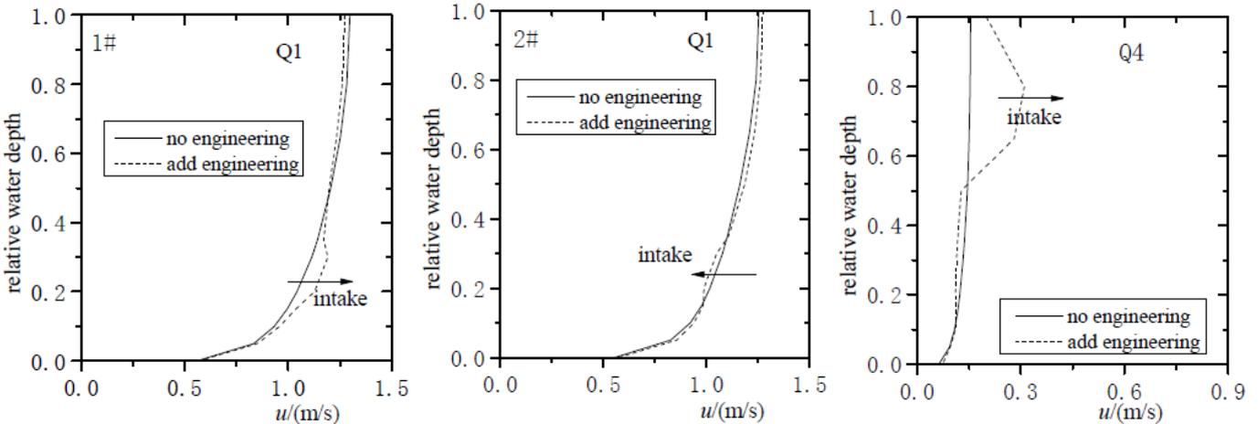
Figure 5. The change of velocity distribution around the intakes.
