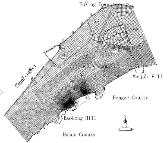
Figure 2. Plane view of grid division of 3D.
