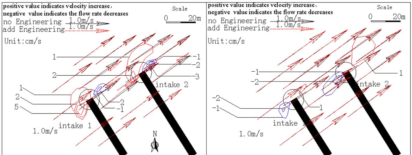
Figure 3. Velocity variation around the intake of design 1.
