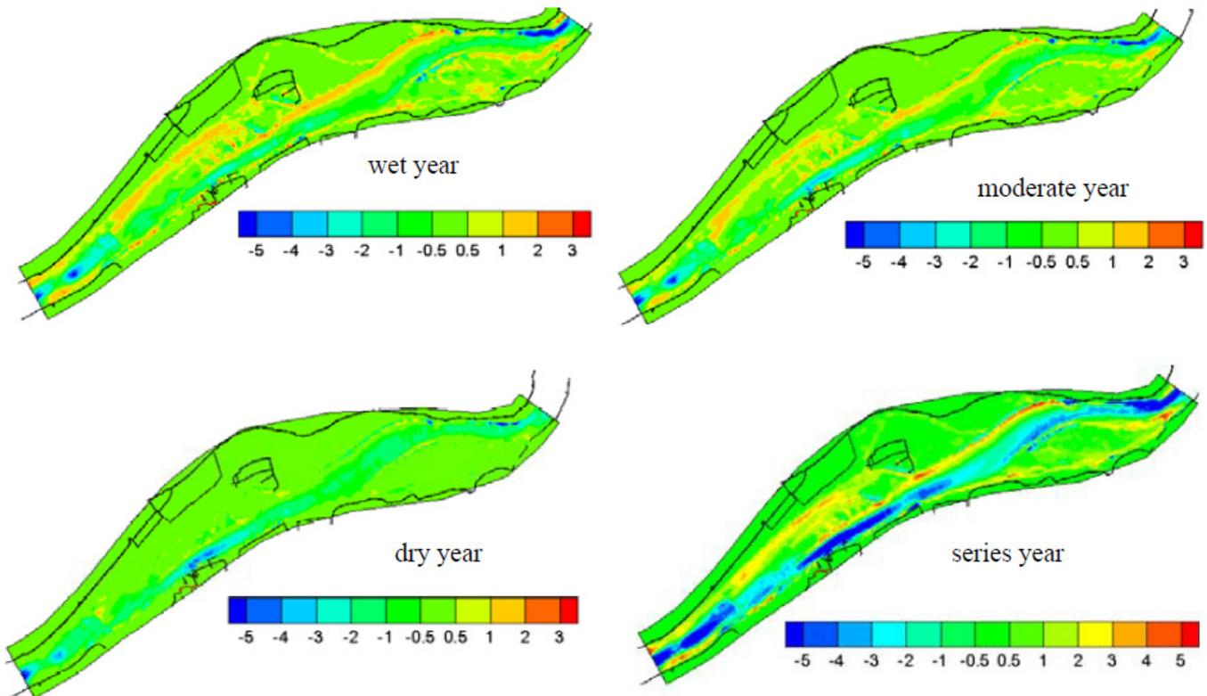
Figure 6. The erosion-deposition distribution in different conditions.
