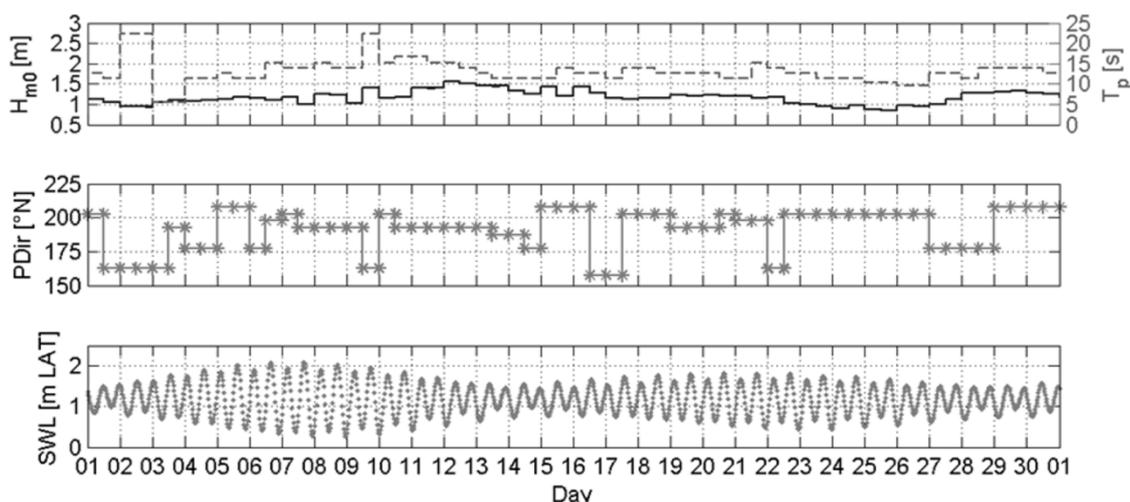
Figure 4. Example of boundary conditions for the XBeach model. Top: wave conditions ( $H_{m0}$  (bold line) and  $T_p$  (dashed line)). Middle: peak wave direction. Bottom: astronomical tide (still water level).
