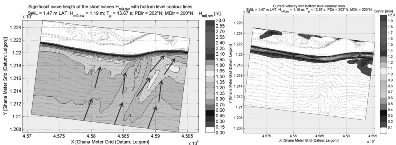
Figure 6. Left: significant wave height  $H_{m0}$  [m] of the short waves for typical wave conditions on background of bottom contour lines (gray dashes, 0.5 m increment). Schematic indication of the wave direction (black arrows). Right: wave-induced longshore current velocities. Schematic indication of the longshore direction and gradient (black arrows).
