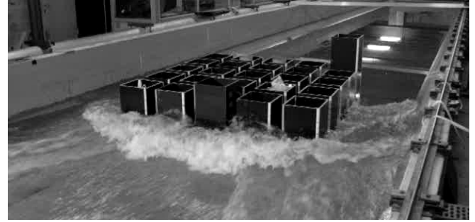
Figure 5. Hydraulic jump upstream of the urban district in transient case
