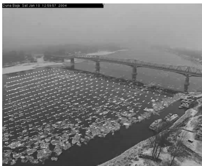
Figure 5. PIV-reconstructed surface velocity vector field
