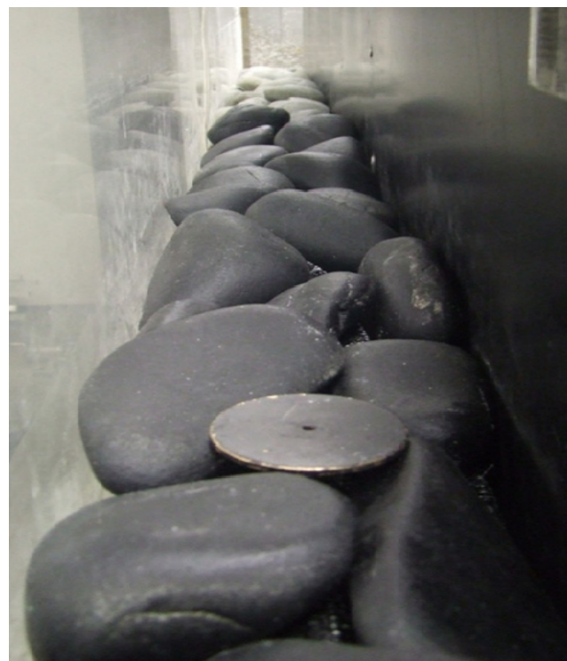
Figure 3. Typical bed configuration showing sensor plate.
