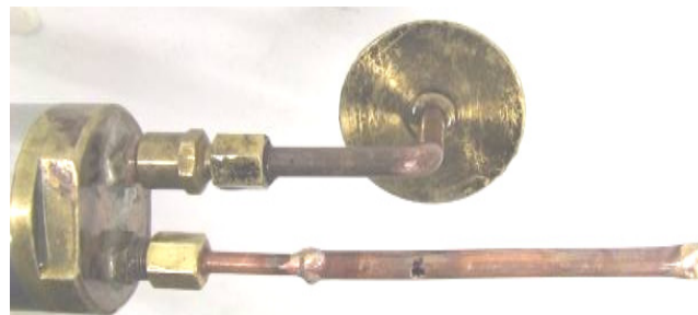
Figure 2. Under-view of pressure ports. The in-bed pressure port is a 3mm hole in a 6mm copper pipe and the bed-plane sensor port is a 3 mm hole (not visible) at the centre of a 50 mm circular plate. This figure is distorted by perspective.
