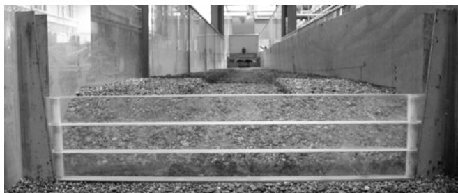
Figure 2. Initial configuration (run 3) with the 3 slats that are to be removed and the small pilot channel.
