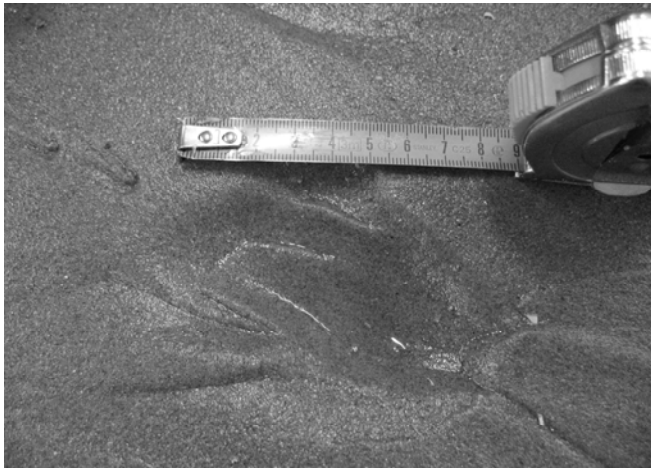
Figure 2. Scour hole in 0.2 mm sand. Flow depth was a few mm while scour depth is a few cm. Ruler in cm for scale.
