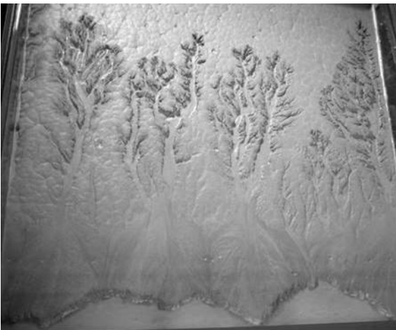
Figure 1. Observed drainage patterns for the 8.5% experiment (top) and for an additional experiment with the same initial planar slope but initial outlet elevation coinciding with the base level (bottom).
