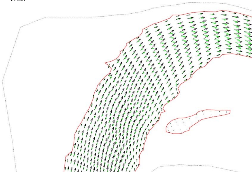
Figure 6. Velocity vectors at the surface (black) and the bed (grey), showing secondary currents in the bend
