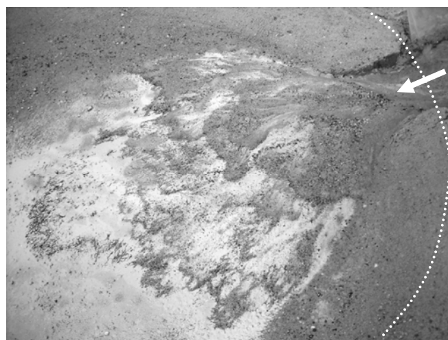
Figure 7. Thin layer of fine sediment draped over the deltaic deposit in the crater lake basin. Note the distinct elongate nature of the individual lobes, brought on by the increase in channel cohesion. Flow from right to left, with low discharge, and 20 % volumetric percentage of silica flour mixed with river sand.
