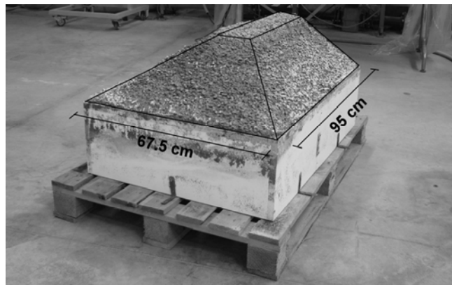
Figure 6. View of the rigid groynes.
