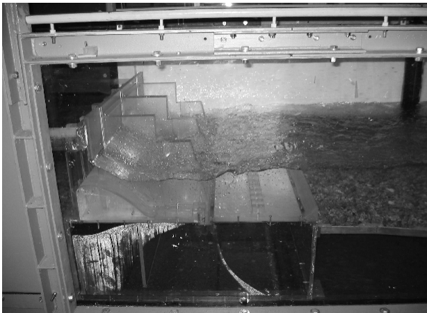
Figure 3. Submerged hydraulic jump for Test Condition 5 with free orifice flow and stable riprap.
