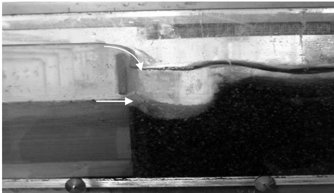
Figure 9 Scouring downstream of combined flow over the weir and under the gate
