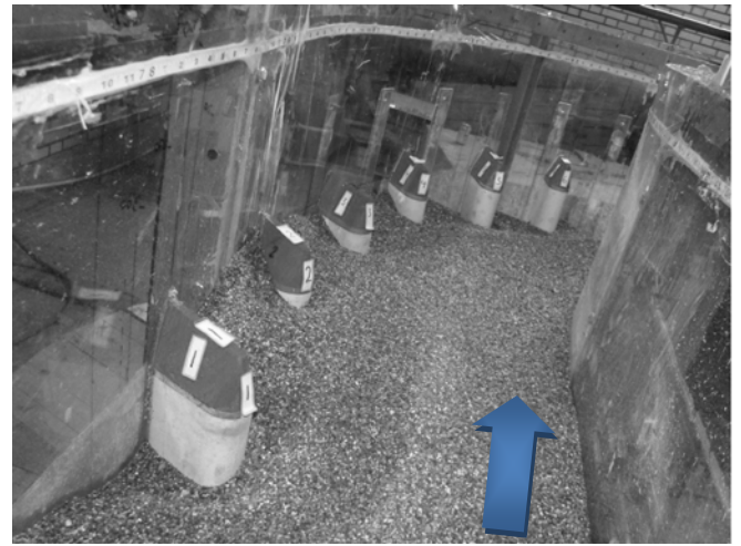
Figure 6 Bendway weirs at 3L spacing and Froude number equal to 0.3(looking downstream)
