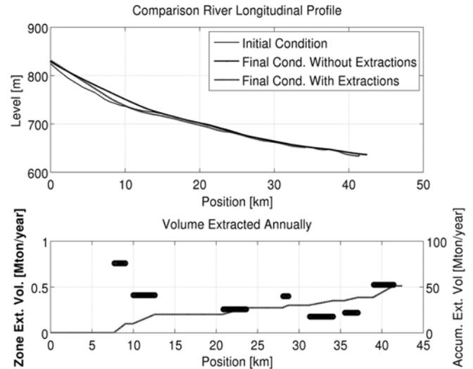
Figure 9. (Upper panel) Comparison between the base case without extraction and the best extraction scenario obtained. (Lower panel) Recommended aggregates extraction rates: DOT – Annual volume of aggregate extracted in zone. LINE – Accumulated volume of aggregate extracted along the river.
