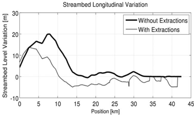
Figure 8. Longitudinal variation of the streambed for cases with and without sediment extraction.
