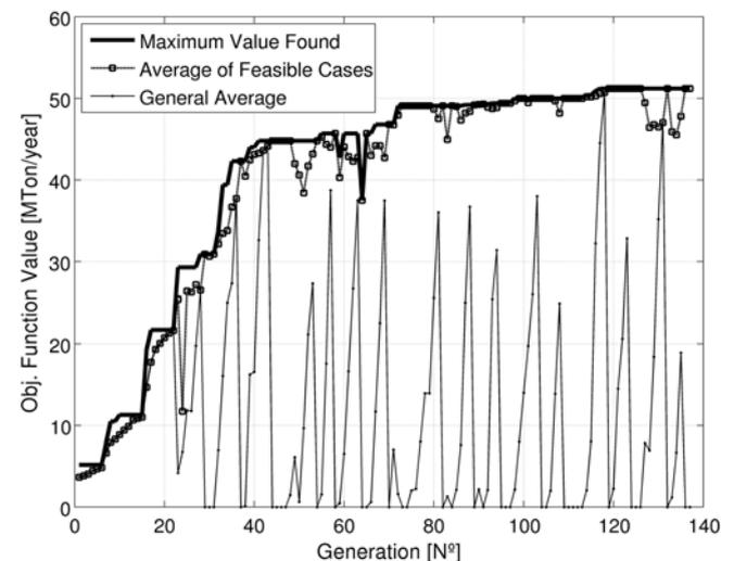
Figure 7. Objective function evolution in terms of the generation number. The feasible average corresponds to the mean of feasible cases that respect the degradation constraints. The general average corresponds to the mean of all the cases. Also the maximum value found in each generation is shown.
