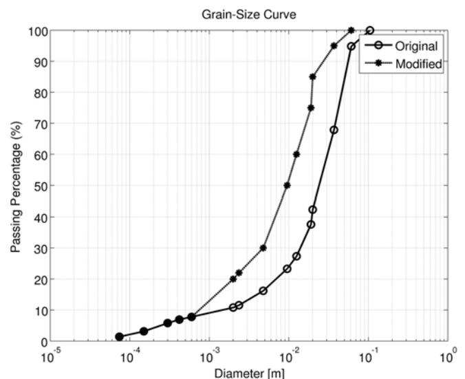
Figure 6. Original and modified grain-size distribution curves for the upper part of Maipo River.
