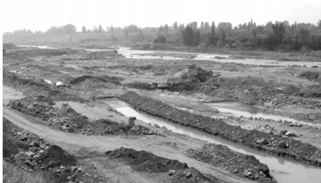
Figure 2. Pit for gravel extraction in the Maipo river. The photograph shows a section of the Maipo river located in the municipality of San Bernardo.
