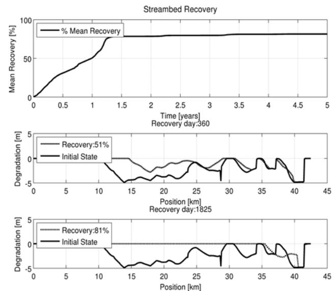
Figure 10. Streambed recovery evolution in time. (upper panel) Mean streambed percentage recovery in time. (middle panel). The recovery is around 51% in day 360. (lower panel) The recovery is around 81% in day 1825 (5 years).
