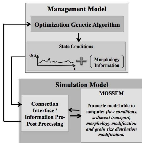
Figure 3. Connectivity implementation between the numerical model (MOSSEM) and the management model.
