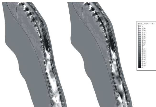
Figure 11. Modeled evolution of nodes within the fairway before (left) and after (right) dredging was initiated (Glander et al. 2009)
