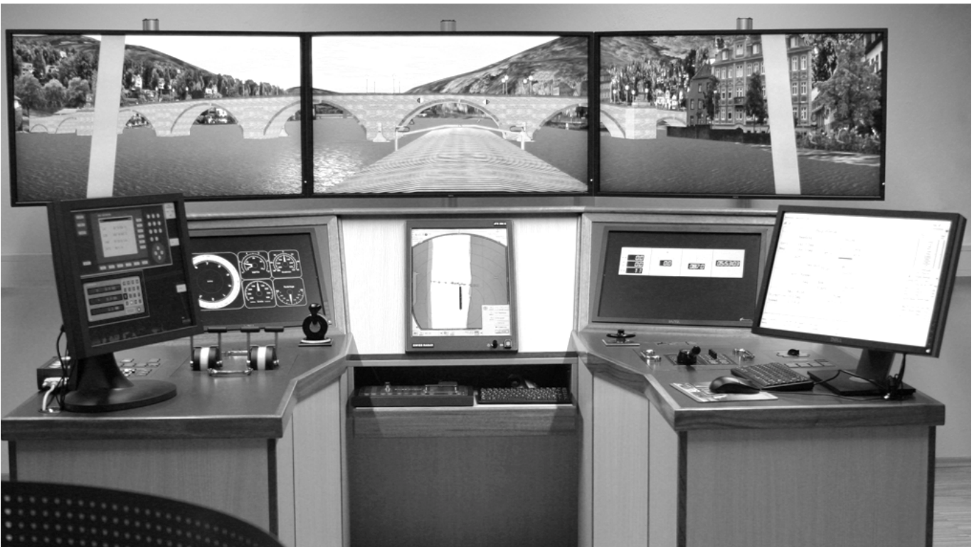
Figure 9: Ship handling simulator, ship-bridge with view scene of the River Neckar at Heidelberg
