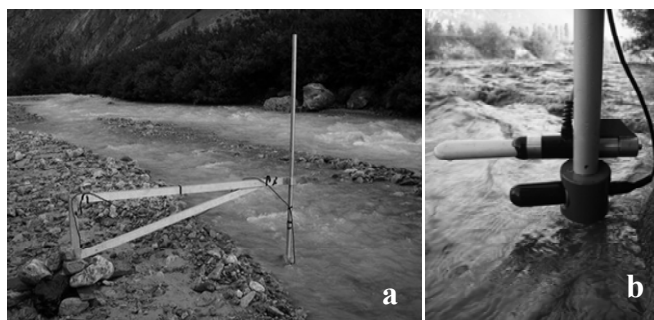
Fig.1a – The hydrophone held by a fixed frame in a mountain creek. Fig.1b – The hydrophone on the frame before immersion. In this experiment, an electromagnetic flow sensor is also used (above). During recordings, the set is oriented upstream.
