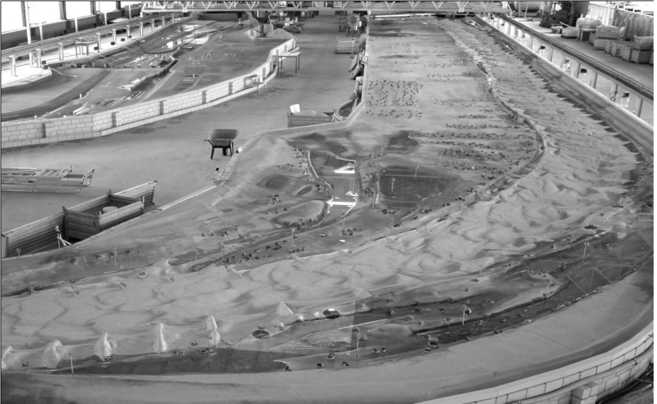
Figure 3: Physical model of the River Oder with the measurement bridge in the background.
