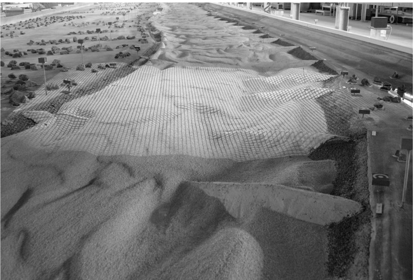
Figure 4: Measurement grid projected onto the model bed.
