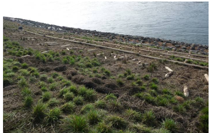
Figure 4: Test field with plant mats arranged on different filter mats
