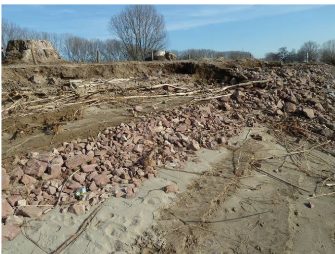
Figure 9: Structural diversity (floating wood debris, different substrates (sand, gravel fill, stones), and break-off edges after flooding in the test field left without bank protection.
