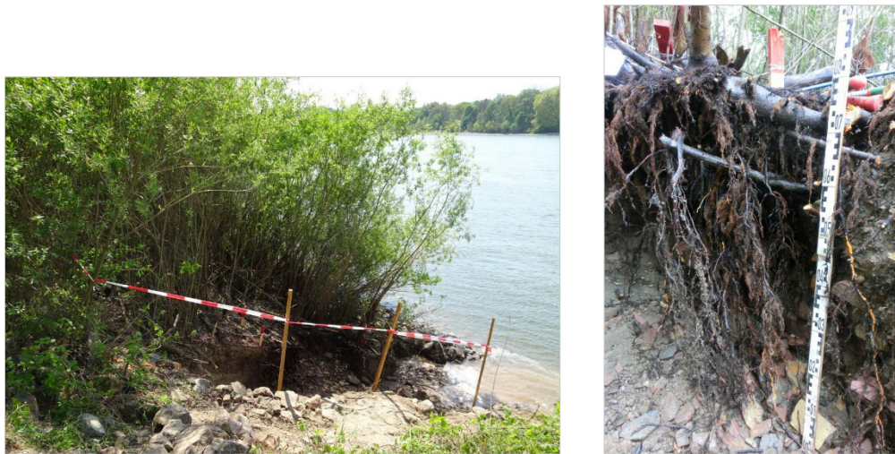
Figure 14: Exposed roots of willows in TF 3 (photos: BAW)
