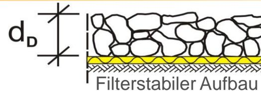
$$\gamma'_D d_D \geq \frac{\Delta u \tan \varphi' - c' - \tau_F}{\cos \beta \tan \varphi' - \sin \beta} - \gamma'_F d_F - \gamma' d_{krit}$$
