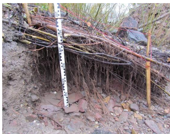
(11) Result of an excavation of roots: root lengths of up to 60 cm in Nov. 2012
