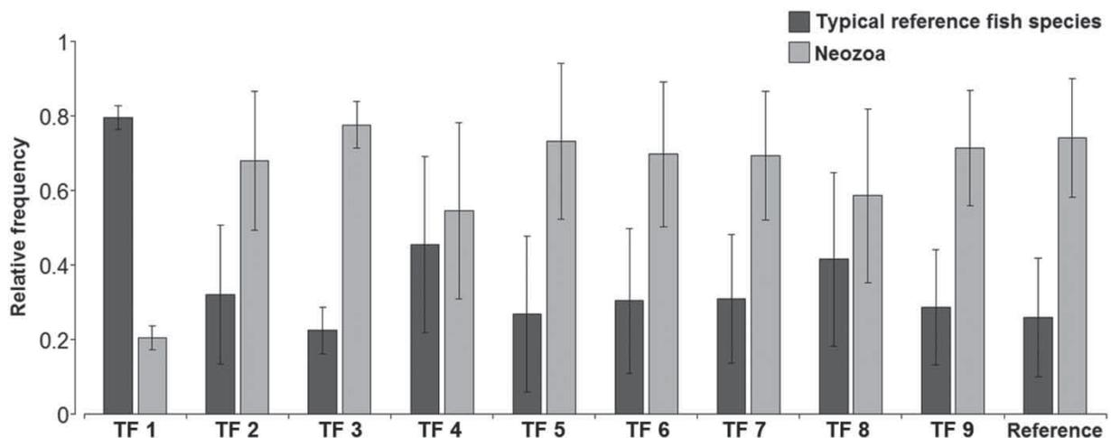
Figure 5. Relative frequency (%) of native fish species and neozoa within the test fields (TF) on the Rhine with (TF1 and 4) and without ecological enhancement (TF2, 3, 5–9) at mean water level compared to the riprap reference.
