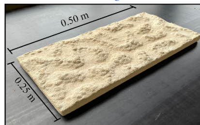
Figure 16: A) Side view and B) cross-section schematics of the experimental setup in the wave flume (not to scale), where SWL denotes the still water level. The positions of the Vectrino Profiler (VP) and wave gauges (WG) are indicated. C) Tiles of the complex M. edulis bed and the M. gigas reef surrogate models are shown exemplarily. Adapted from Hitzegrad et al. (2025b).
