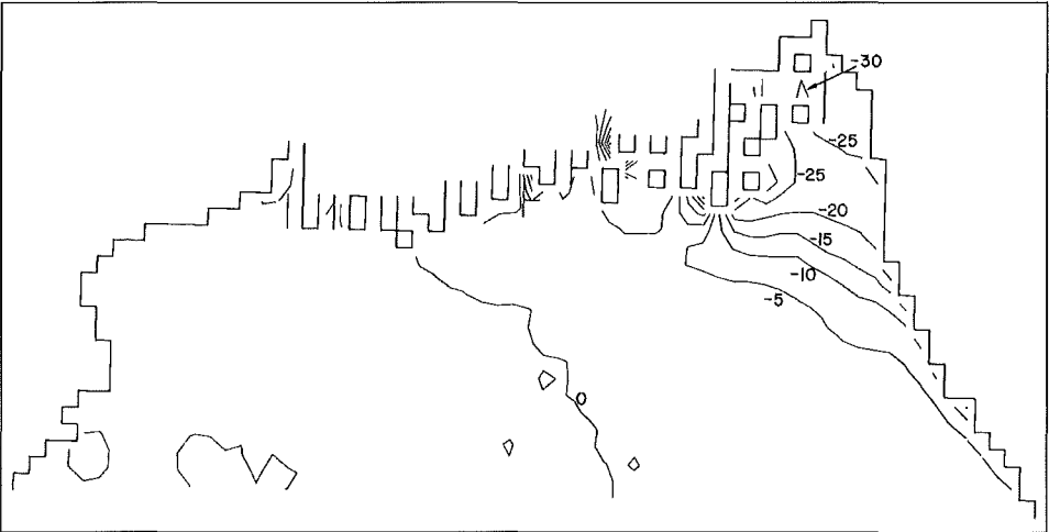
Fig. 8.7(b): Change (cm) in maximum computed elevation (cm) produced by a 2 m rise in MSL (FLATHER and KHANDKER, 1993)
