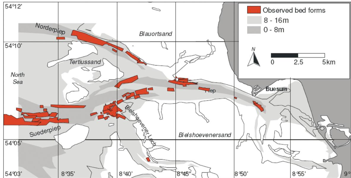
Fig. 7: Regions where bed forms were observed, also indicating the thickness of the potentially mobile sediment layer above the EHL
