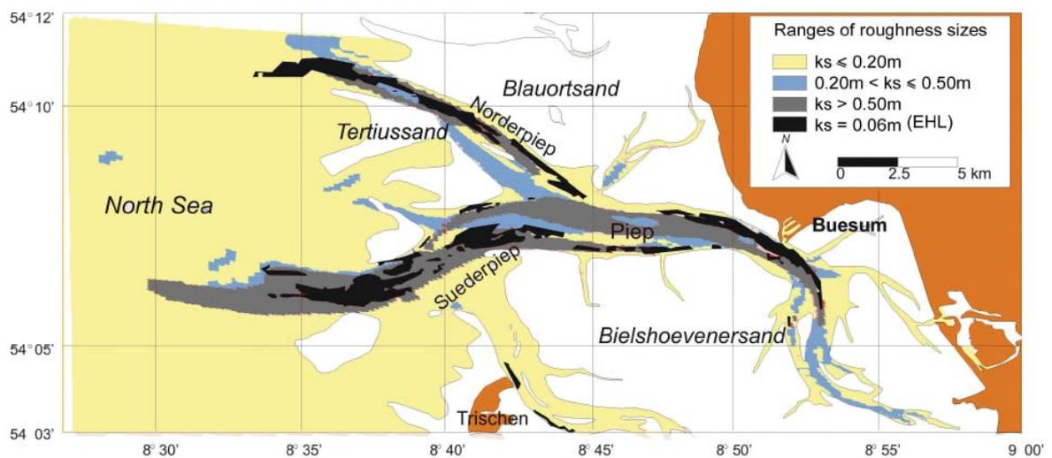
Fig. 17: Roughness values computed using empirical equations
