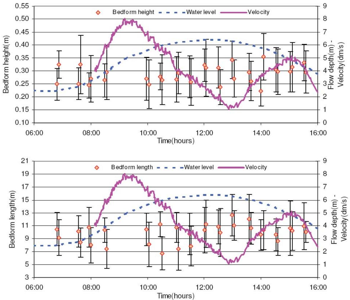
Fig. 10: Temporal variation of bed-form dimensions in the inner Piep tidal channel; upper: bed-form heights; lower: bed-form lengths
