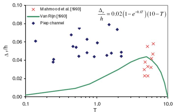
Fig. 13: Relative bed-form heights of megaripples after VAN RIJN (1993)
