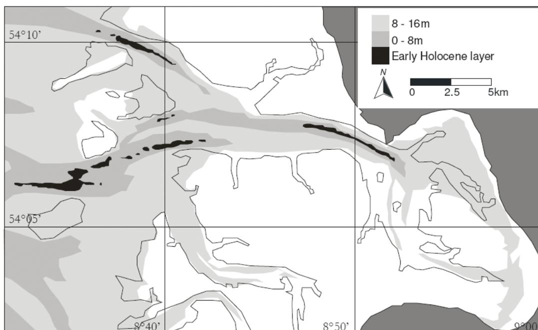
Fig. 2: Thickness of the potentially mobile sediment layer above the EHL (modified after ASP, 2004)
