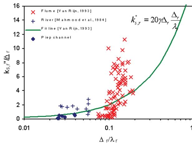
Fig. 14: Relative form roughness of megaripples after VAN RIJN (1993)
