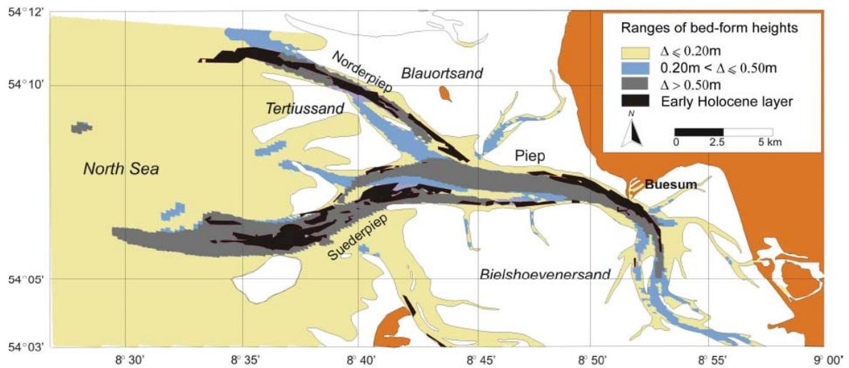
Fig. 15: Predicted heights of bed forms in the tidal channels for a spring tide
