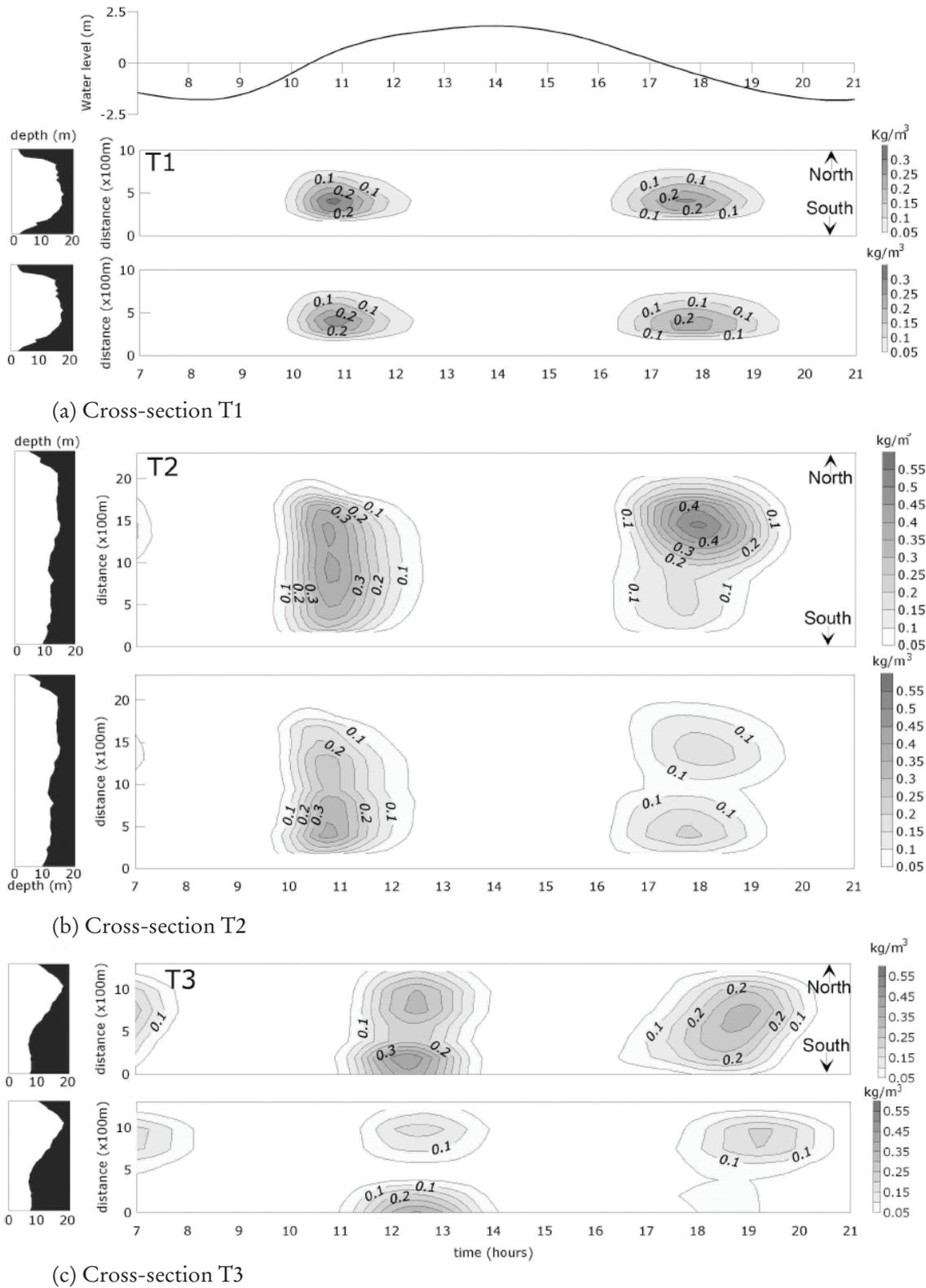
Fig. 20: Influence of bed roughness on the computed variation of depth-averaged suspended sediment concentration for a spring tide at cross-sections T1, T2 and T3. Upper plot: constant Chezy coefficient; lower plot: predicted bed roughness
