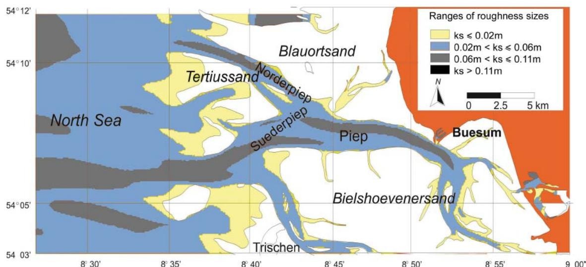
Fig. 18: Roughness values based upon a constant Chezy coefficient of  $60 \text{ m}^{1/2}/\text{s}$
