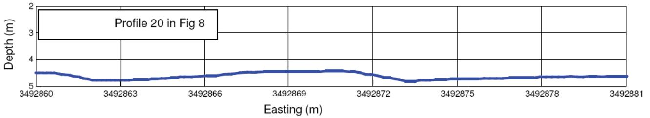
Fig. 9: Typical bed-form feature without scale distortion in the inner Piep tidal channel
