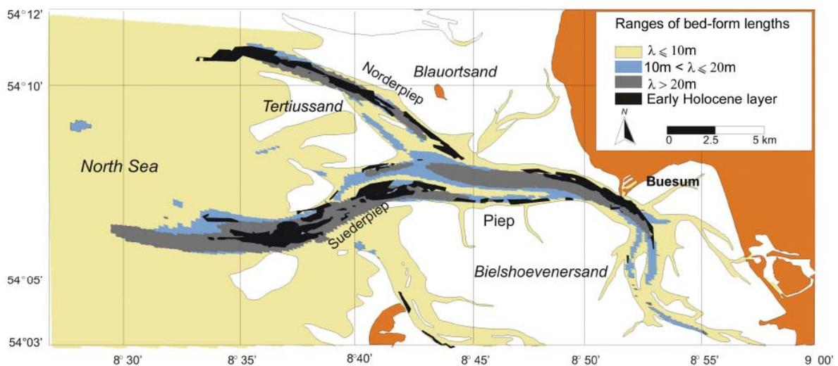
Fig. 16: Predicted lengths of bed-form features in the tidal channels for a spring tide
