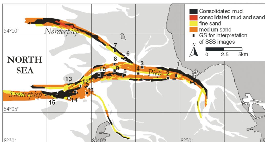
Fig. 3: Surficial seabed sediment distribution in the main tidal channels (modified after VELA-DIEZ, 2001)
