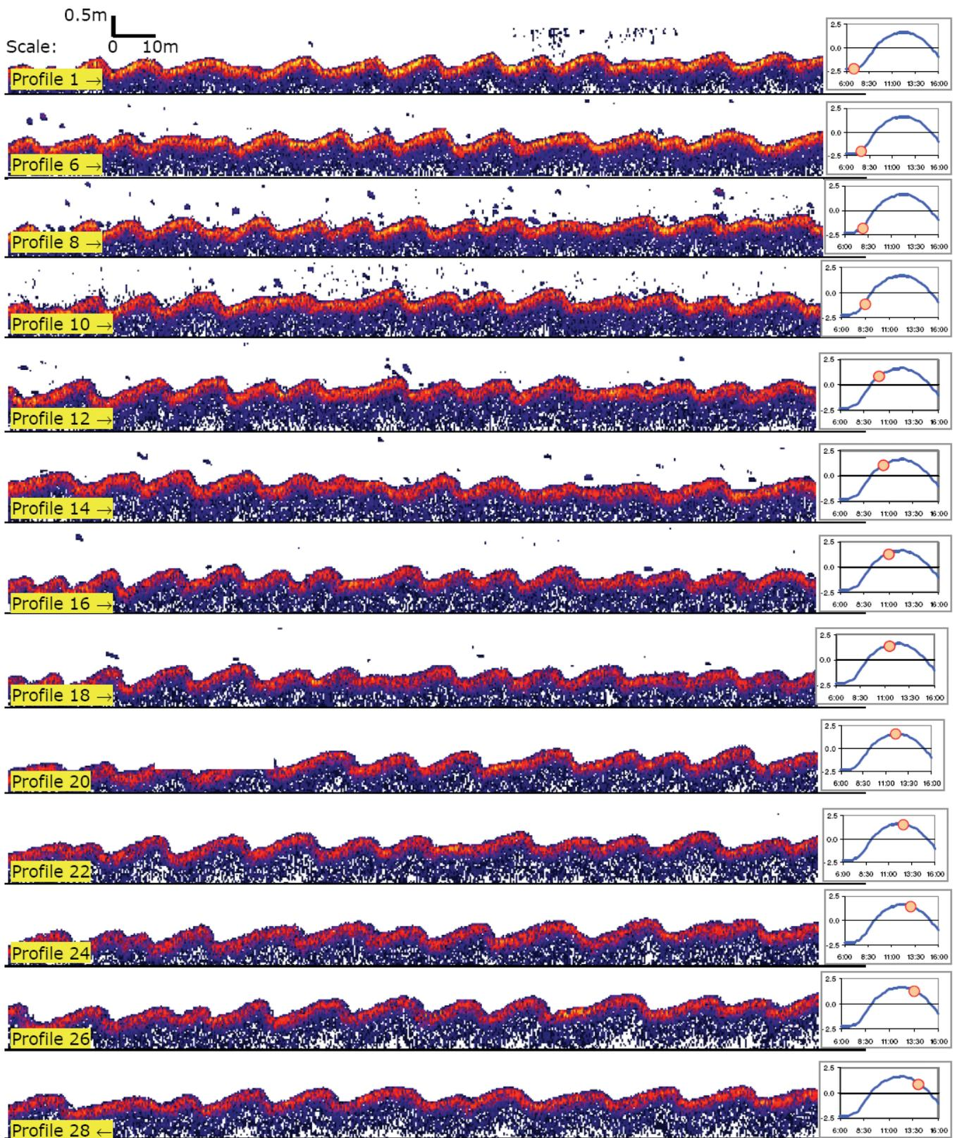
Fig. 8: Measured bed profiles with exaggeration of the vertical scale in the inner Piep tidal channel
