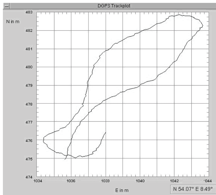
Fig. 1: Example of a local measurement; duration: 240 sec, mean flow velocity: 20 cm/s; local stability could only be attained over an area of 10 \times 10 metres; the figure was obtained by running DSLP-software during measurements
