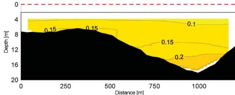
(d) Suspended material concentrations in  $\text{kg}/\text{m}^3$  estimated using DEINES' approach
