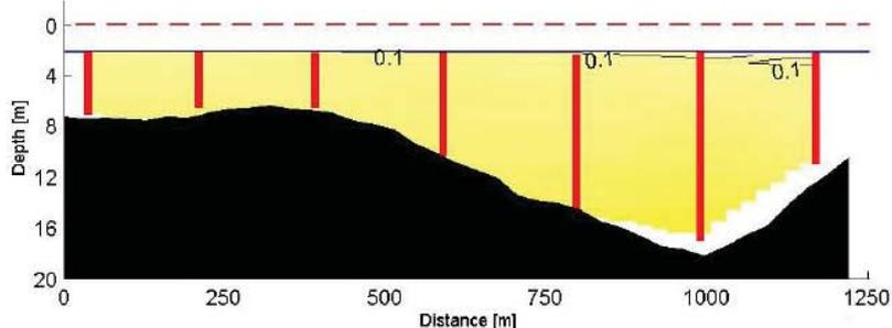
(b) Suspended material concentrations in  $\text{kg}/\text{m}^3$  obtained from optical transmission conversion
