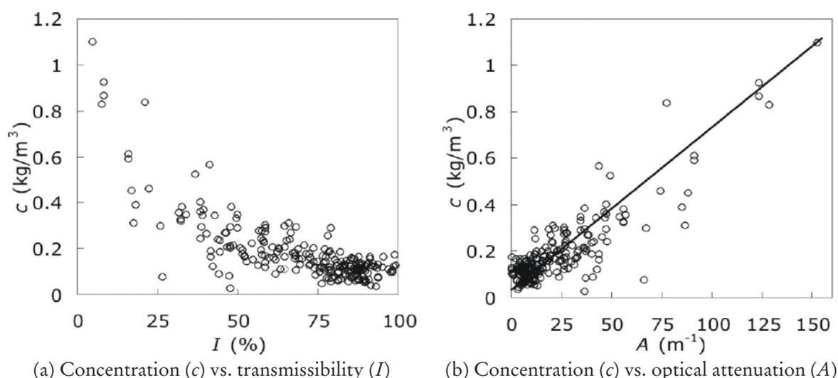
Fig. 2: Calibration of optical concentration measurements
