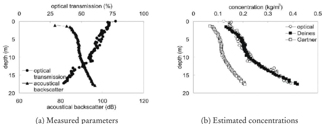
Fig. 8: Profile measurement in cross-section T3 during maximum flood flow on 23 March 2000
