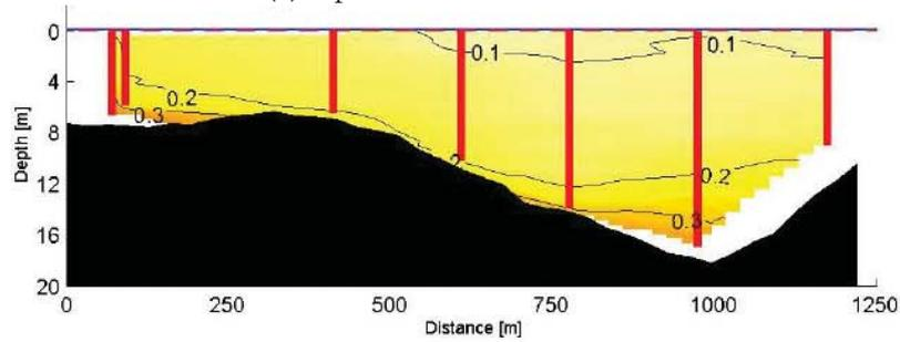
(b) Suspended material concentrations in  $\text{kg}/\text{m}^3$  obtained from optical transmission conversion
