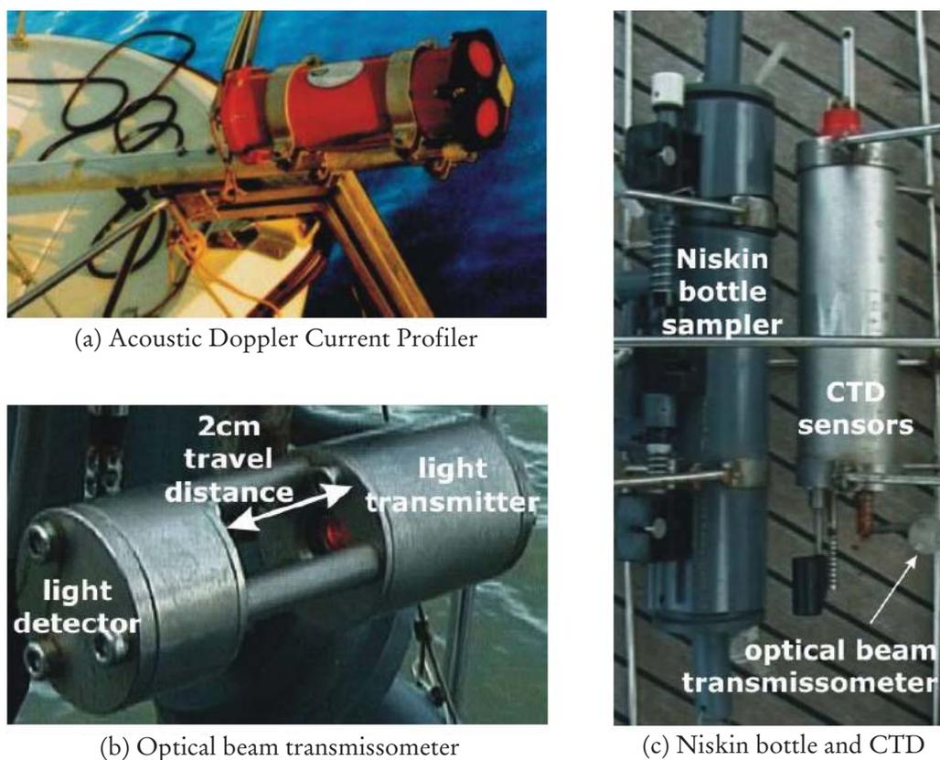
Fig. 1: Measuring devices used in the study
