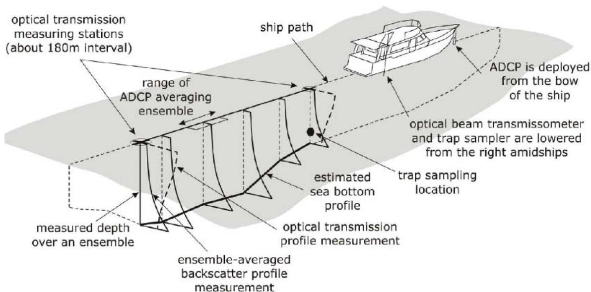
Fig. 4: Measurement procedure
