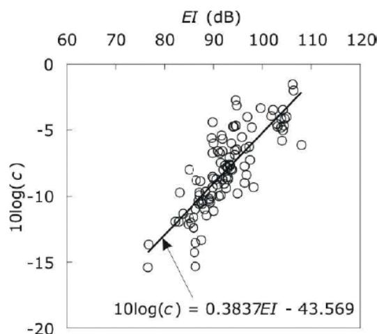
Fig. 5: Independent backscatter calibration based on direct sampling concentrations
