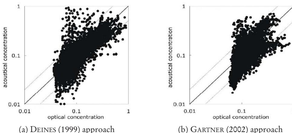
Fig. 6: Comparison of optical and acoustic concentration measurements in kg/m<sup>3</sup>
