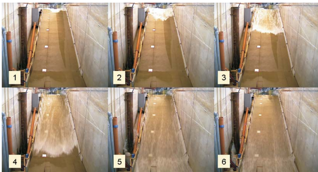
Fig. 5.40: Overtopping flow on the landward slope (Large Wave Flume, Hannover) (photo: SCHÜTTRUMPF)
