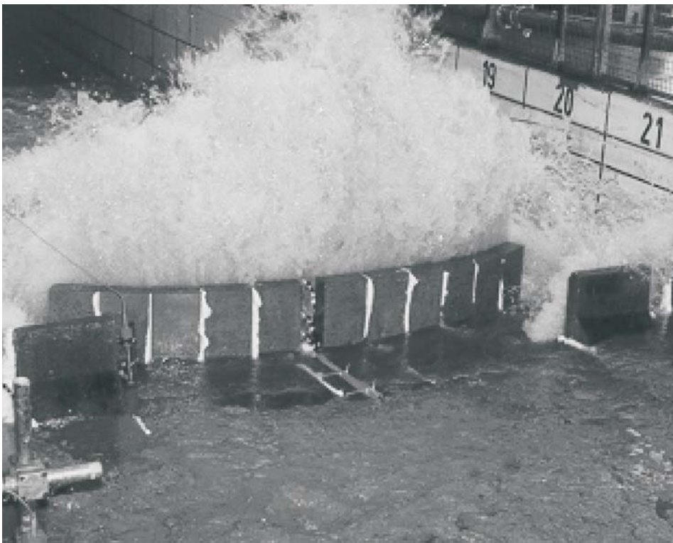
Fig. 5.31: Influence of a wave wall on wave overtopping (photo: SCHÜTTRUMPF)
