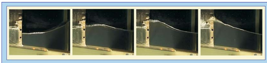
Fig. 7.3: A non-impulsive (pulsating) wave condition at a vertical wall, resulting in non-impulsive (or “green water”) overtopping
