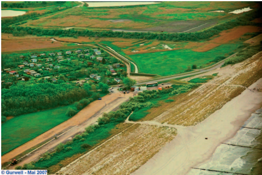
Fig. 5: Groins, beach nourishment, dyke and steel wall in Markgrafeneheide
