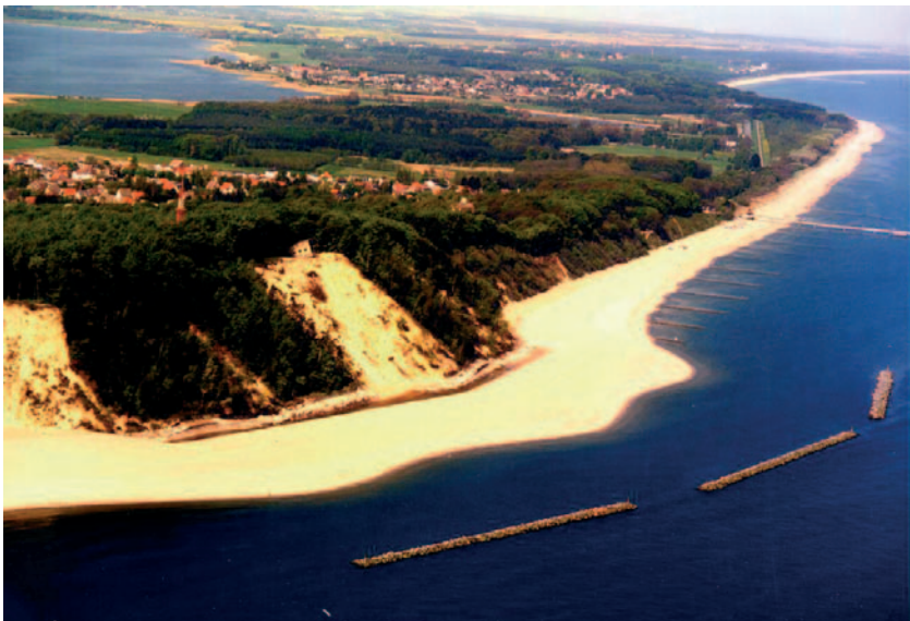
Fig. 4: Breakwaters and sea wall on the Island of Usedom
