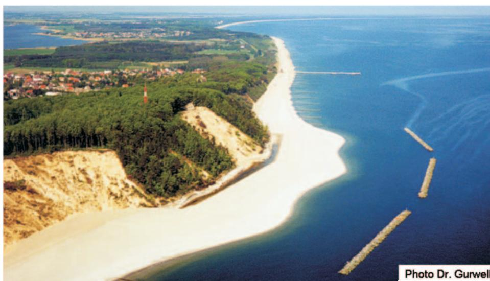
Fig. 8: System of detached breakwaters at Streckelsberg/Usedom
