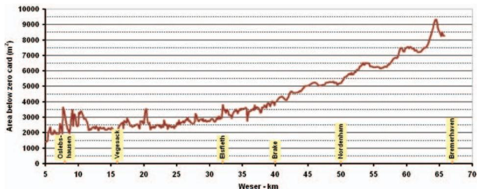
Fig. 4: Cross-sectional area below reference datum along the Lower Weser
