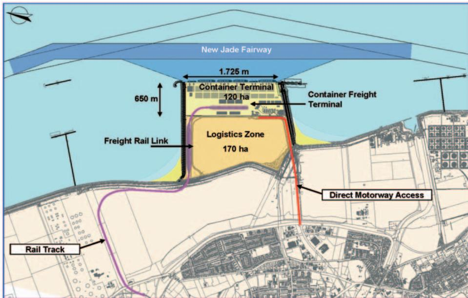
Fig. 4: The port and its modified access channel
