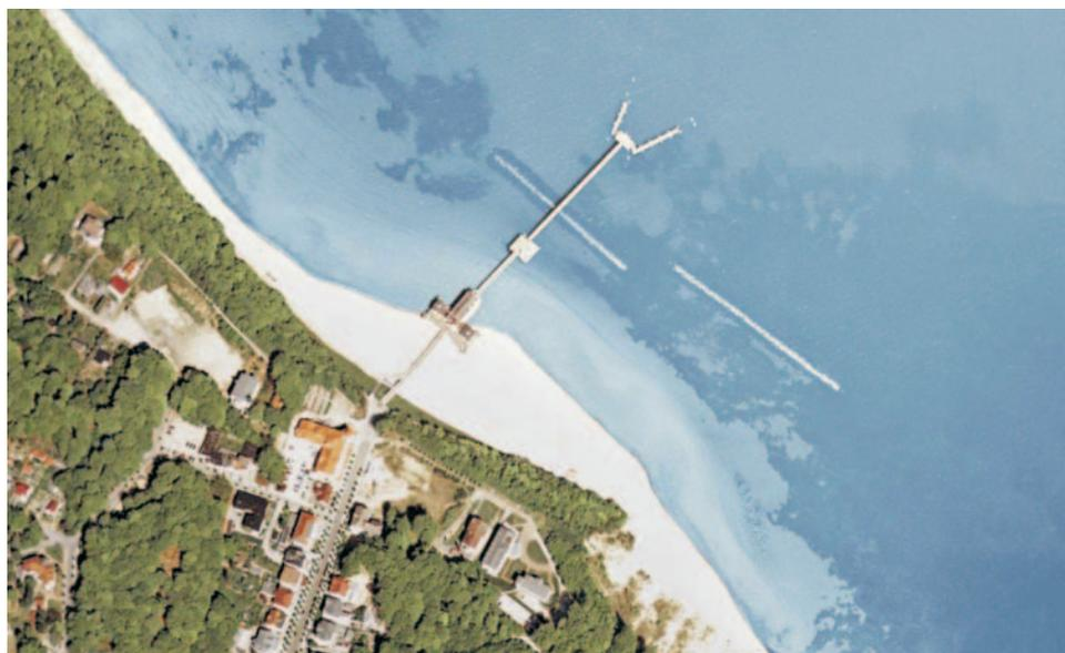
Fig. 3: System of detached breakwaters at Sellin/Rügen (Google Earth)
