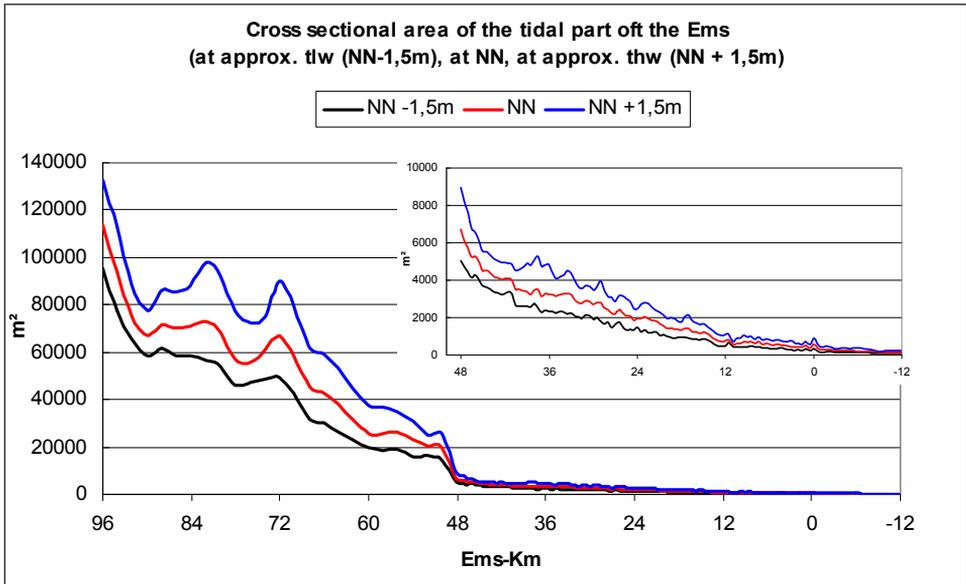
Fig. 2: Present cross-sections in the Ems Estuary as a function of the distance to the geographic origin of the system (tidal boundary)
