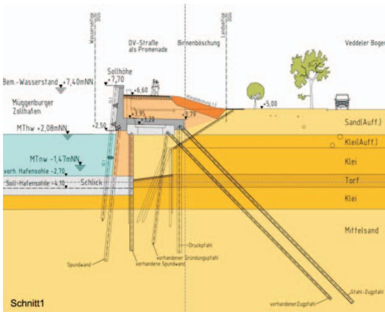
Fig. 2: Example of combined cantilever retaining wall (Hamburg)
