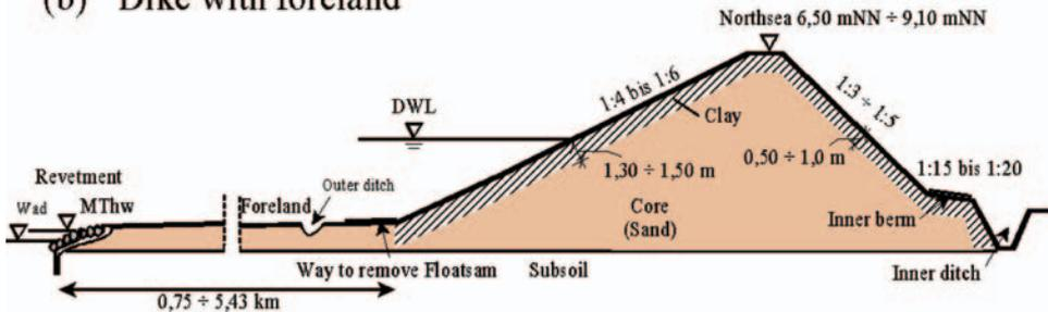
Fig. 5: Typical dike profiles in Germany (SCHÜTTRUMPF, 2001)
