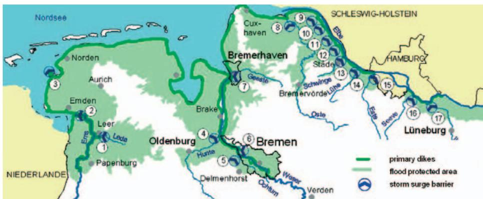
Fig. 3: Overview over primary dikes, storm surge barriers and flood protected area in Niedersachsen. (1) Leda barrier, (2) Ems barrier, (3) Barrier Leysiel, (4) Hunte barrier, (5) Ochtum barrier, (6) Lesum barrier, (7) Geeste barrier, (8) Oste barrier, (9) Barrier Freiburg, (10) Barrier Wischhafen, (11) Barrier Ruthenstrom, (12) Barrier Abbenfleth, (13) Schwinge barrier, (14) Lüle barrier, (15) Este barrier, (16) Barrier Seevesiel, (17) Ilmenau barrier
