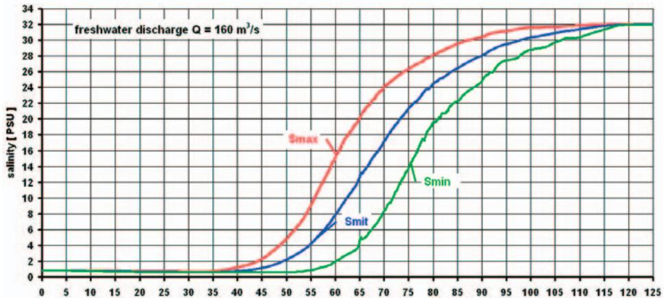
Fig. 9: Location of the brackish water zone at a discharge of  $160 \text{ m}^3/\text{s}$  (num. model investigations BAW)
