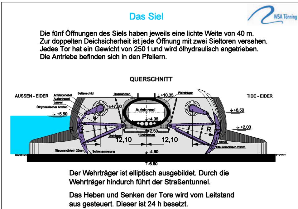
Fig. 9: Cross-section of the barrage/© WSA Tönning
