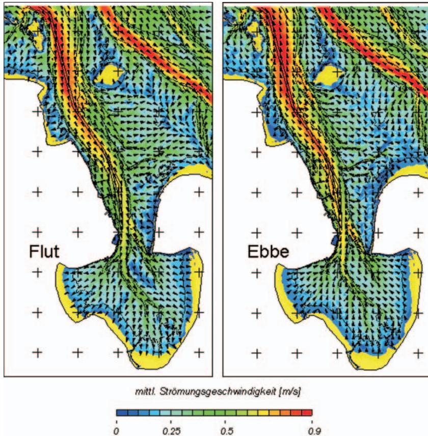
Fig. 5: Flood (right) and ebb (left) current velocities averaged over a neap-spring cycle obtained from a 3D-HN simulation with the model UnTRIM3D (BAW, 2003a)
