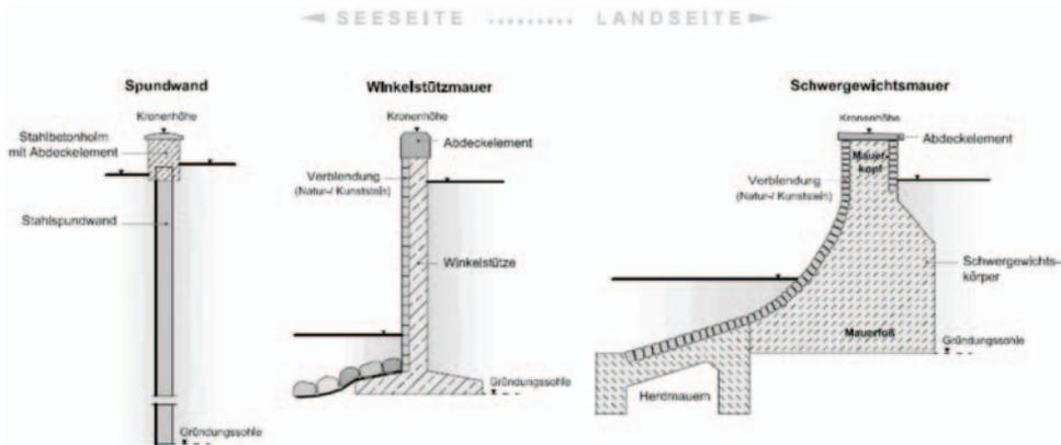
Fig. 1: Examples of storm surge protection walls
