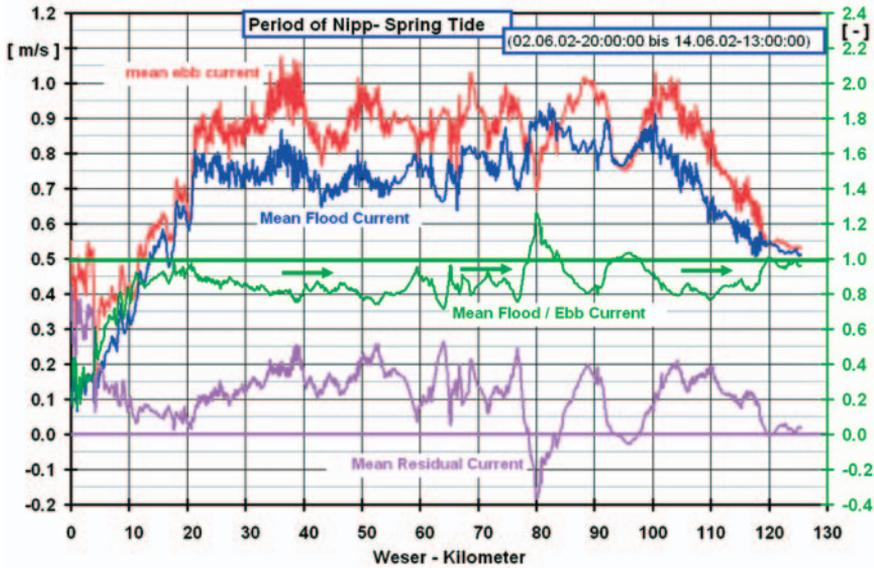
Fig. 10: Longitudinal section of vertically averaged flood and ebb currents during a spring-neap-cycle, of residual currents and of the ratio of flood and ebb current velocity (num. model investigations BAW)
