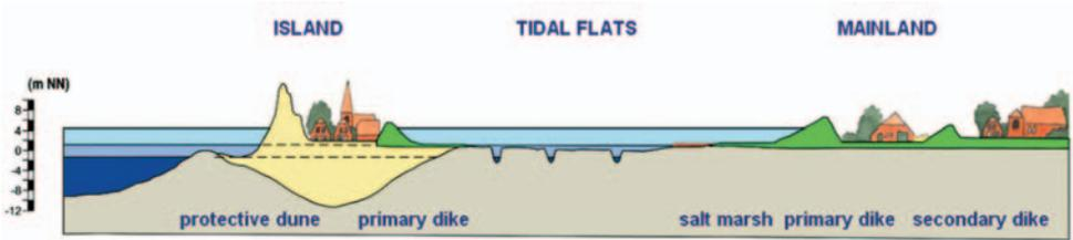
Fig. 4: Coastal flood defence system in Niedersachsen
