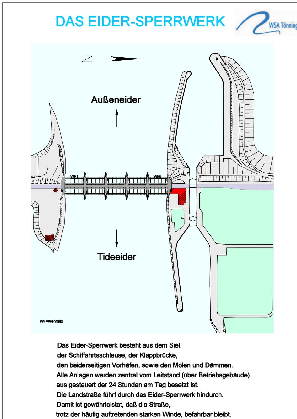
Fig. 10: Layout plan of the barrage/© WSA Tönning
