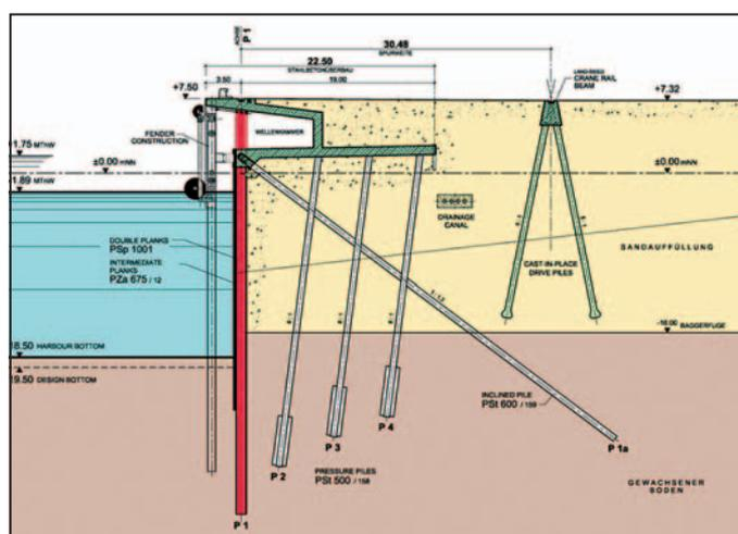
Fig. 4: Cross-section of CT 4 quay wall
