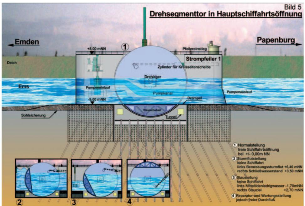
Fig. 3: Cross-section of pier No. 2/© NLWKN Aurich
