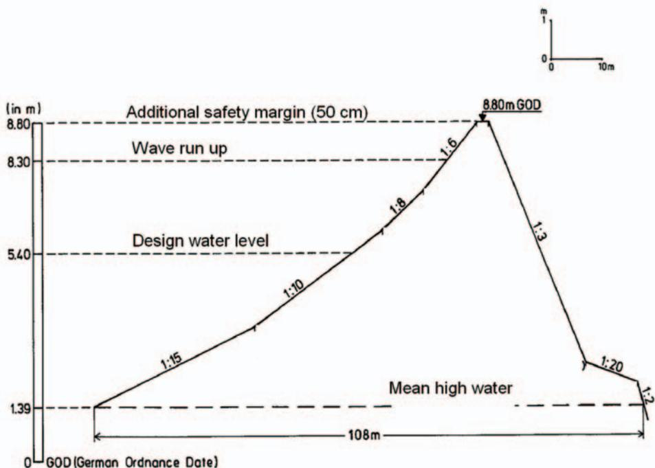
Fig. 3: Dimensions of a state dike (schematic)
