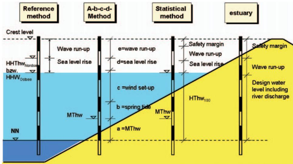
Fig. 6: Methods to calculate the design water level in Germany
