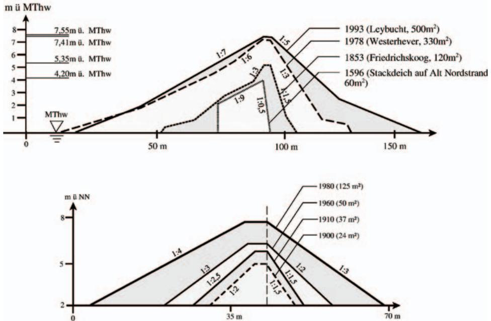
Fig. 2. Evolution of dike profiles in the past (SCHÜTTRUMPF and OUMERACI, 2002)
