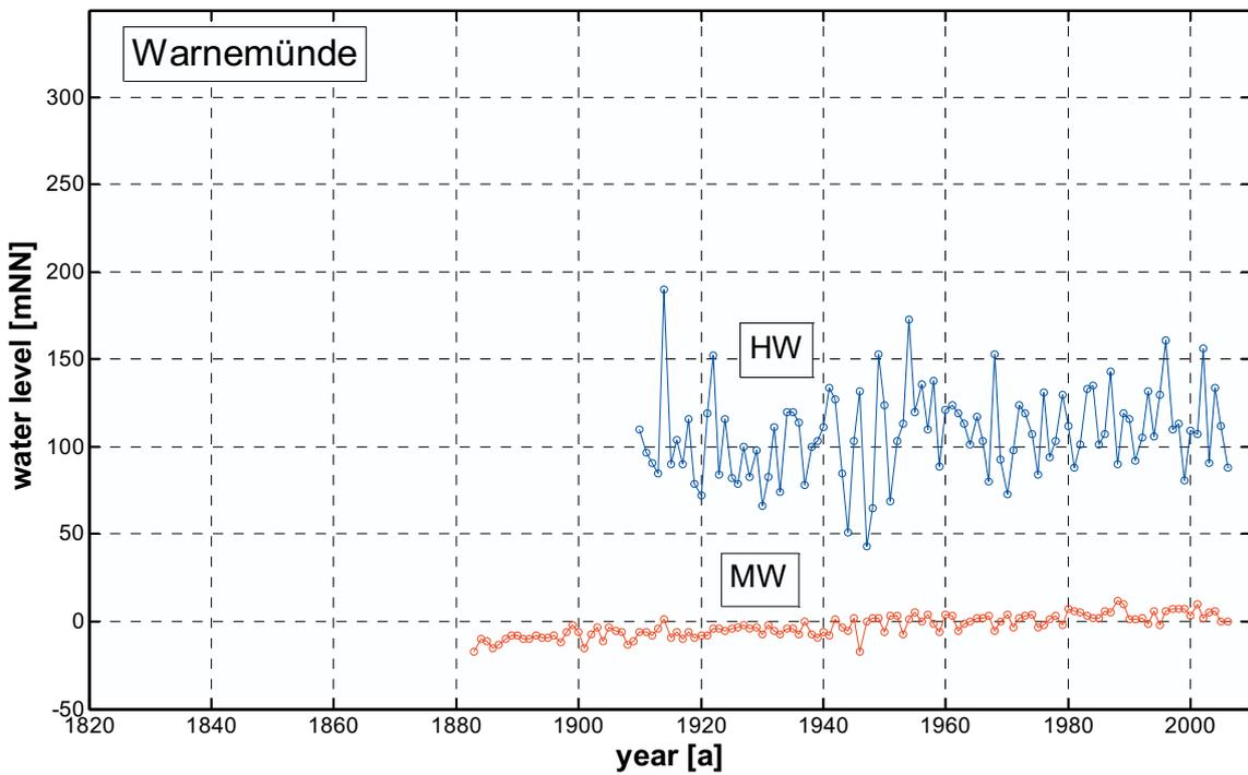
Fig. 5: Time series of mean water and high water levels at the Travemünde and Warnemünde gauge stations
