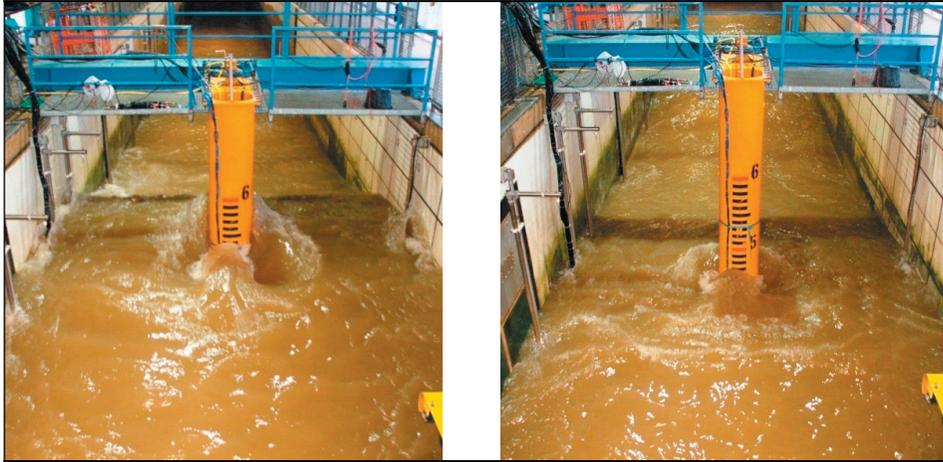
Fig. 44: Complex flow induced by wave/pile interaction
