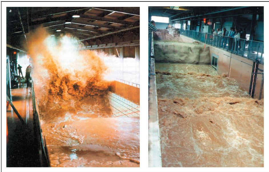
Fig. 48: Beach/dune profile development under extreme wave conditions in the GWK
